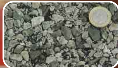
Left: A typical part of one of the marked sections of roads – see the hard self-stabilised lateritic base layer beneath the bitumen surfacing, which has given very good performance Below: A marginal quality silcrete used as surfacing aggregate in Botswana
