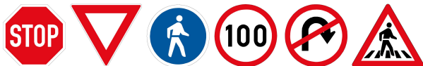
Figure 1: Typical traffic signs, showing their unique colour and shape (from left to right: stop, yield, pedestrians only, 100km/h speed limit, no u-turn, pedestrian crossing ahead) (note that images are available in colour).
