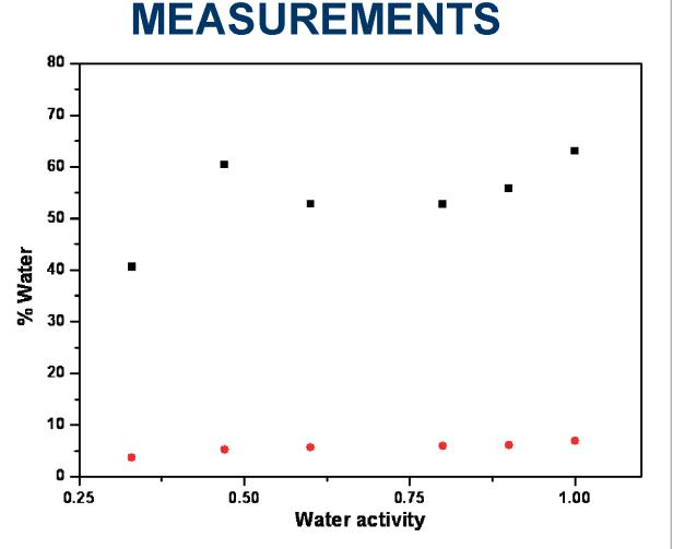
Figure 3: Water sorptions of the thin films of 3b and Nafion at 40 °C using quartz micro-balance [11].
