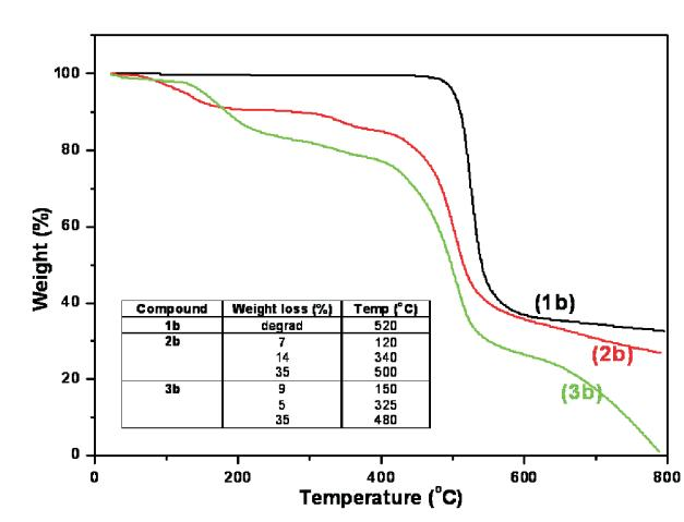
Figure 2: TG curves of compounds (1b), (2b) and (3b). All samples were heated at 10 °C/min under N<sub>2</sub>.
