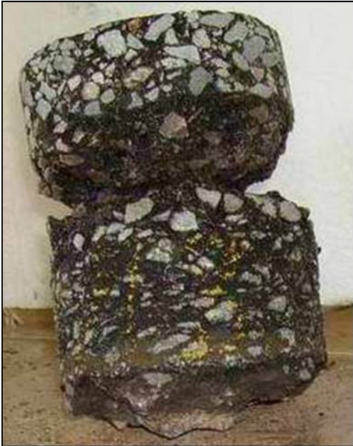
Figure 7: Typical 100mm diameter core from section P3
