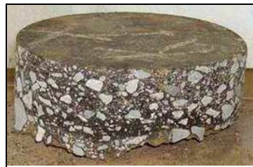
Figure 6: Core taken from the wheel path of section P2
