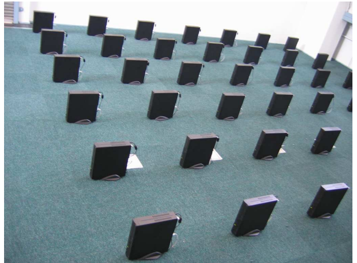
Fig. 6. Layout of the 7x7 grid of Wi-Fi enabled computers
