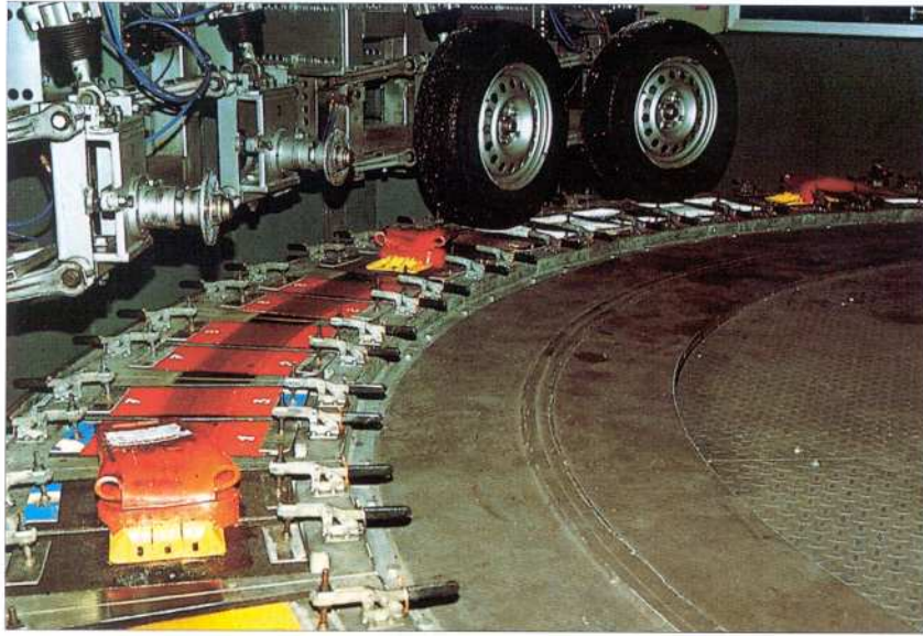
PHOTO 4: Circular Pavement markings test facility
