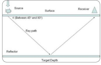
Fig. 1: Schematic diagram of the seismic data acquisitioning process.
