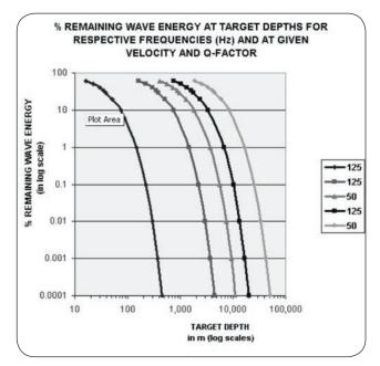
*Fig. 4: Penetration depths as calculated by the spreadsheet.*
