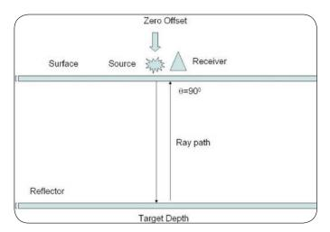
Fig. 2: Schematic of the zero offset principal.
