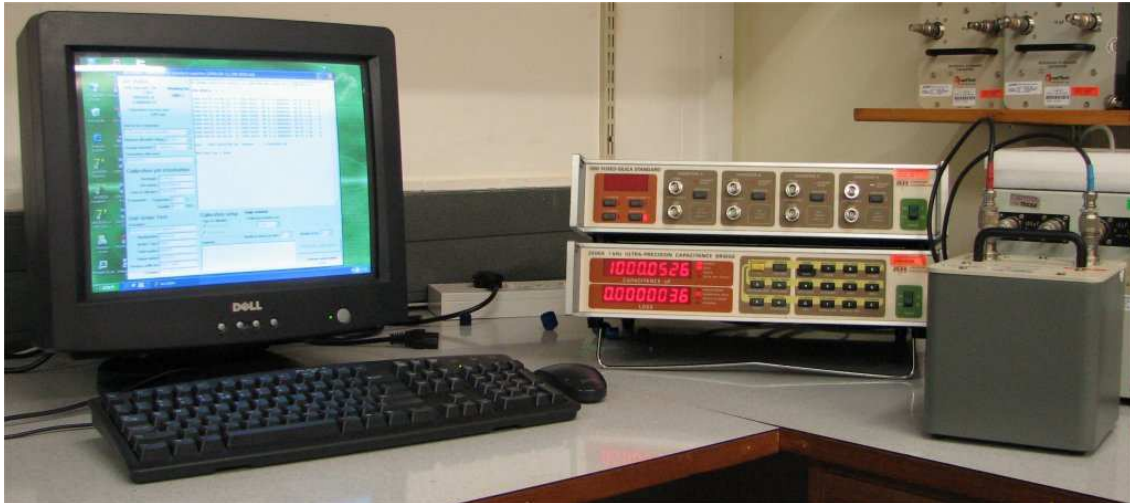
Figure 6: Measurement setup for capacitance calibration.
