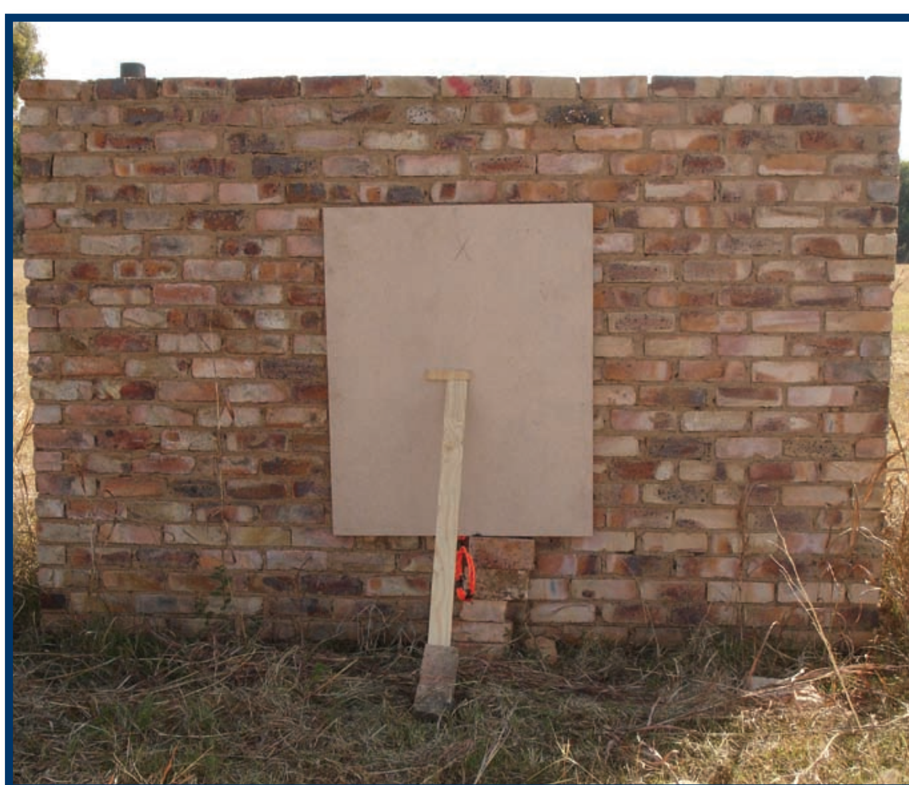
Figure 3. Charge positioned against the brick wall
