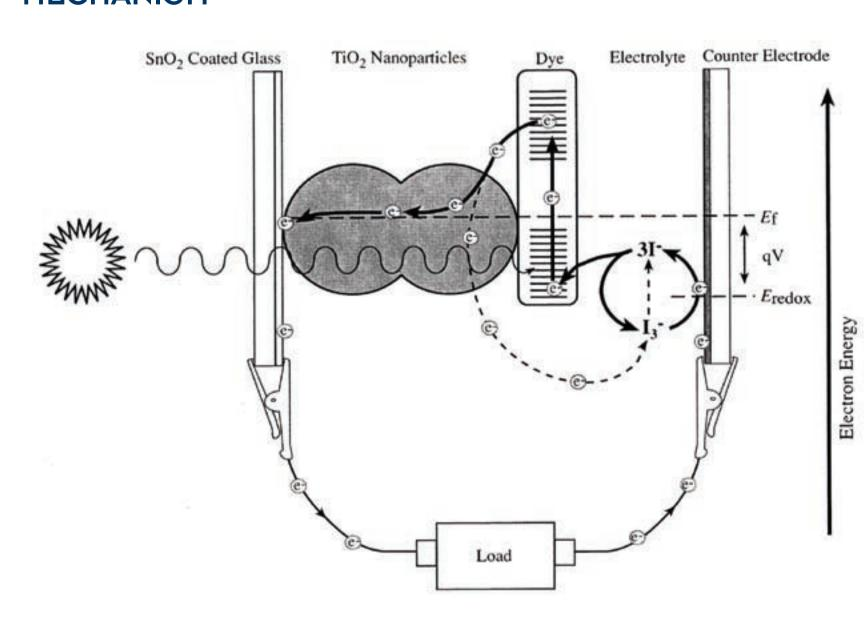
When light enters the cell through the glass substrate, the electrons in the Ru-dye get exited. The active components in these cells are nano-particles of titanium oxide – a semiconductor with a large band gap of 3-3.2 eV. Incident light excites the organic dye molecules on the titanium sites in the nanoporous film. This causes electrons to be released into the semiconductor layer to generate an electrical current. The band gap is too large for the electrons to fall
