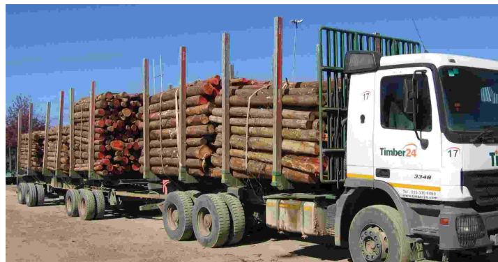
Figure 2. Example baseline vehicle comprising a rigid truck towing a 4-axle drawbar trailer.
