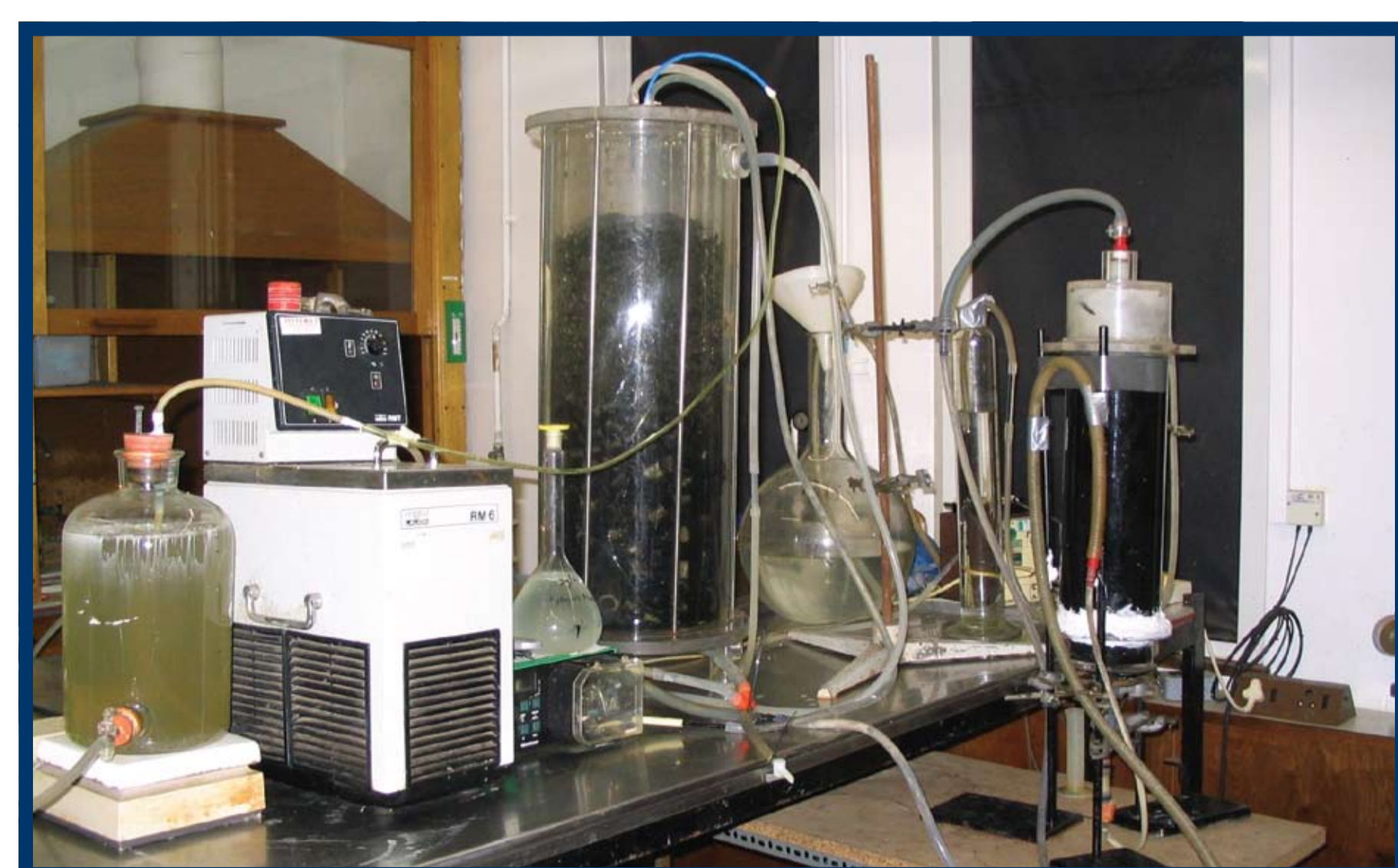
Figure 3: Laboratory scale hybrid reactor system FR
