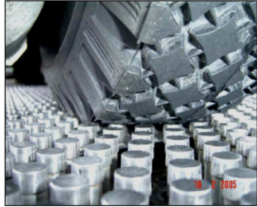
Figure 4. Close-up: 1/3 rd scale square profile (D-tyre) of MMLS3 on the rough-textured (RT) SIM surface.
