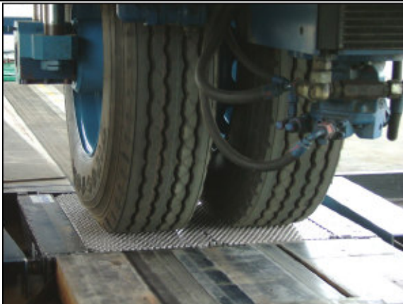
Figure 3. Model Mobile Load Simulator (MMLS3) on the SIM device at Gauteng Department of Public Transport, Roads and Works (GDPTRW) Koedoespoort facility.
