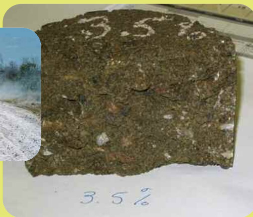
Sample manufactured with 3.5% agribinder, which has properties between conventional asphalt and cement concrete
