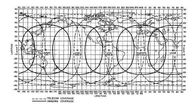
Fig 2.The covering of IDCS satellites. Telecommunication coverage is shown by the dashed lines around each satellite position
