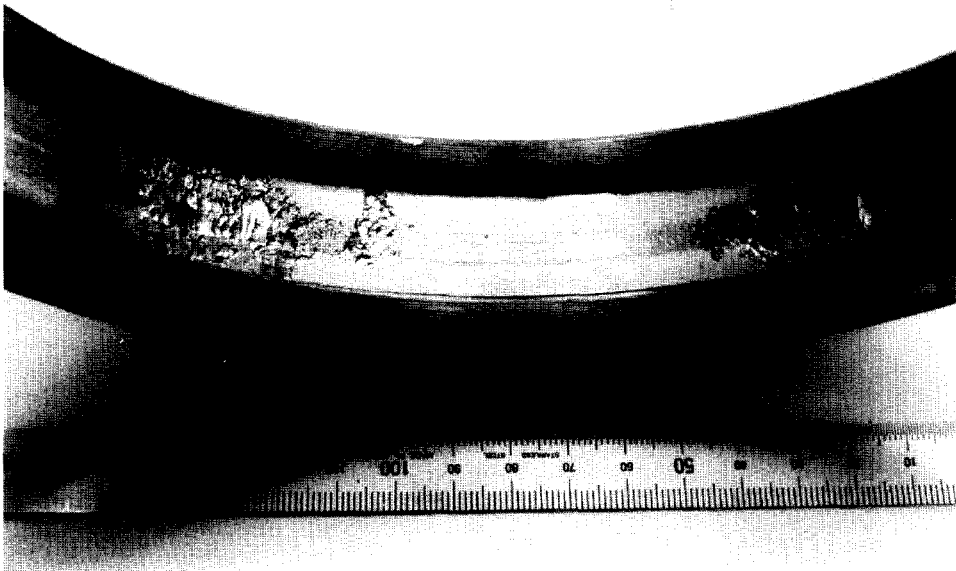
Fig. 5. Flaking damage on the outer raceway of a roller bearing.
