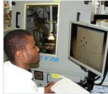
CSIR researcher, Mesuli Mbanjwa, machining with the Excimer laser machining equipment
