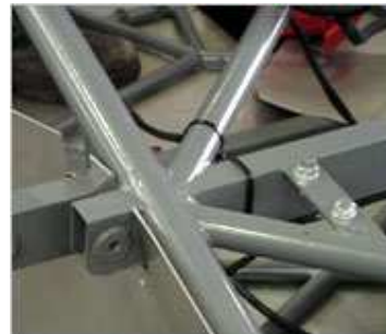
A close-up of a welded frame of one of the replica cars that was laser-cut
