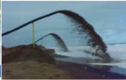
Dredger tailings discharged to the inter-tidal zone on the Namibian coast. Image courtesy: Namdeb Diamond Corporation
