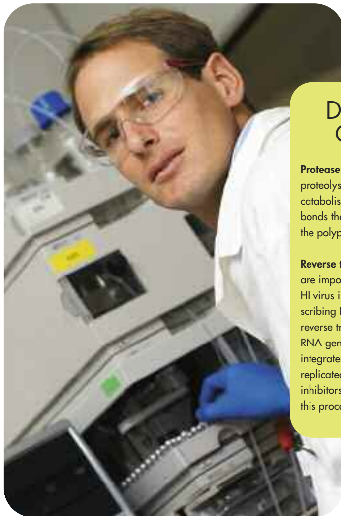
Dr Jaco Zeevaart enjoys technical work like woodwork in his spare time. Here he loads samples in the high pressure liquid chromatography machine for analysis of sample purity
