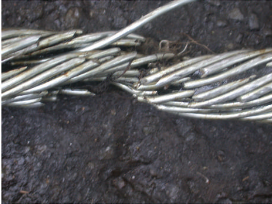
Figure 3.3: Close up of non-spin rope inner strand failure.
