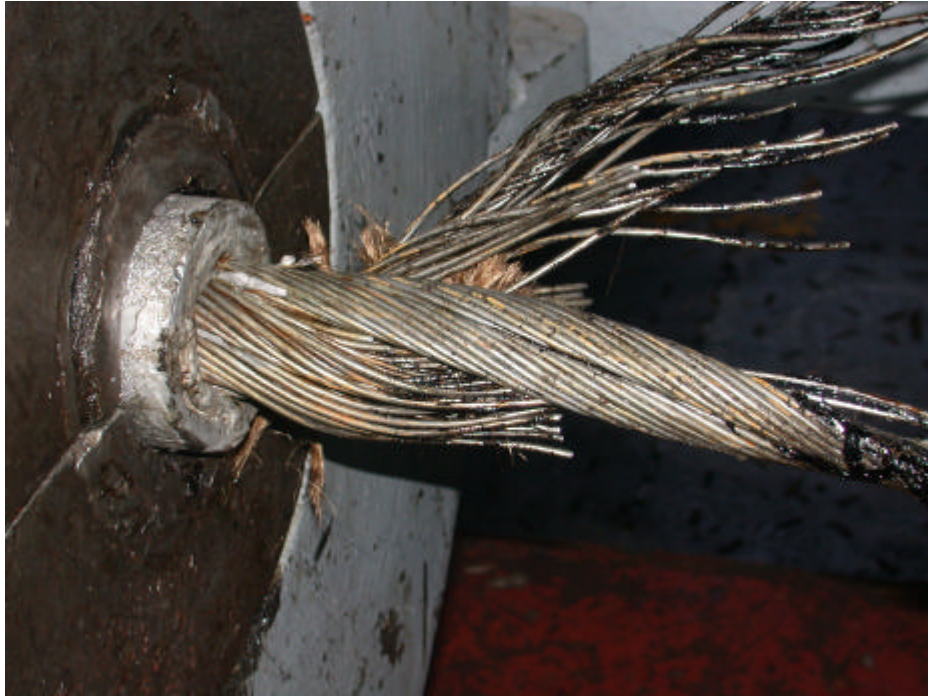
Figure 3.1: End cap break, 2,75 mm triangular strand.
