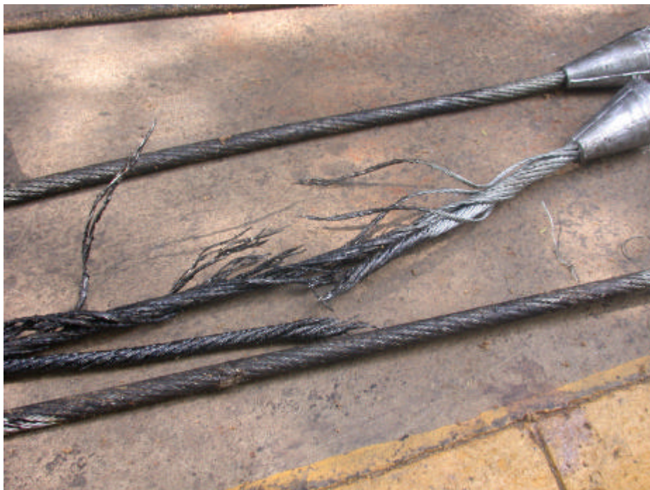
Figure 3.2: Failure of 2,75 m non-spin rope.
