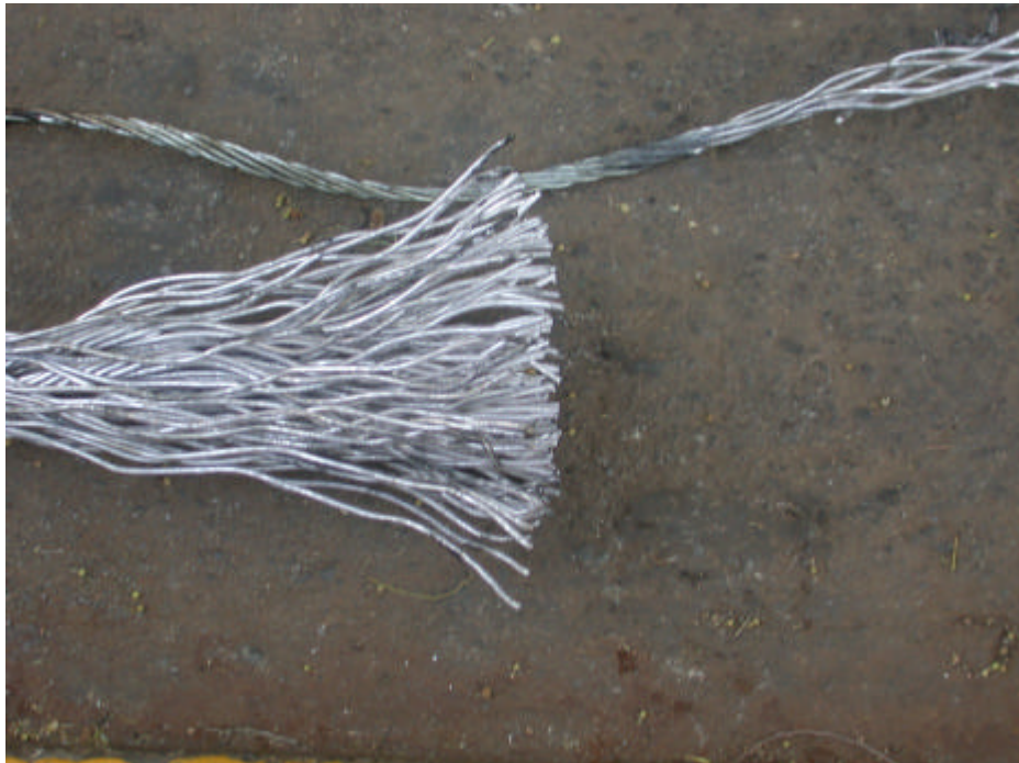
Figure 3.4: Non-spin rope brush.
