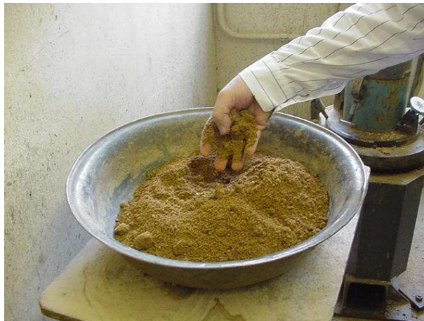
Photograph 3: Four hour lime/slag treated material just before compaction. Notice the loose texture.
