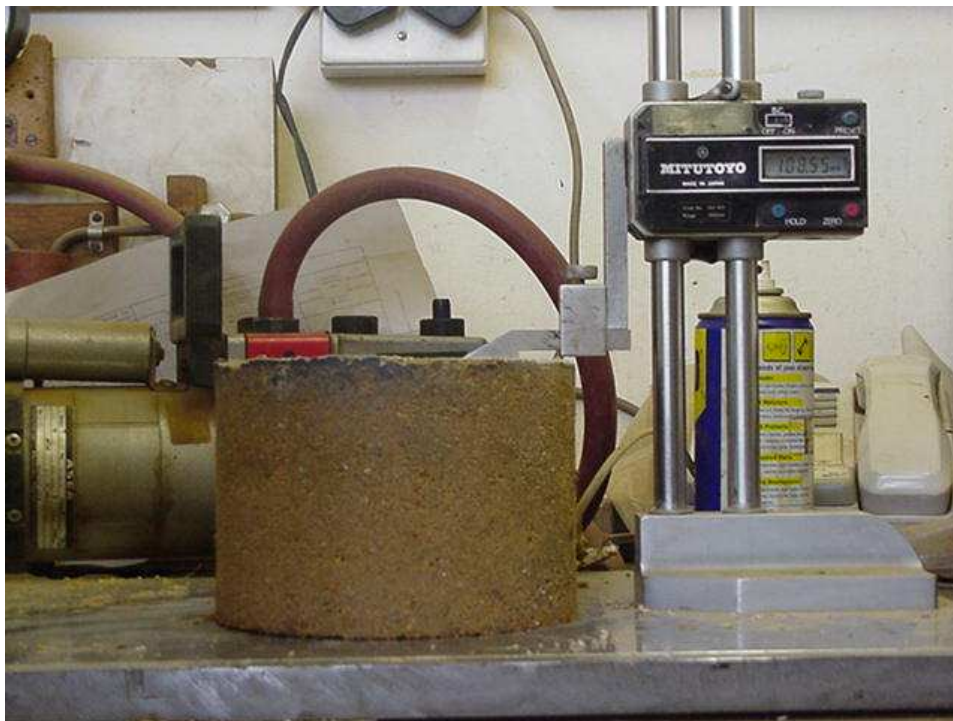
Photograph 6: Measuring height of four hour Builtcrete sample compacted on vibratory table. Notice height reading of 108.55 mm. Sample size was calculated to be approximately 100 mm high when compacted to 100% Mod.AASHTO
