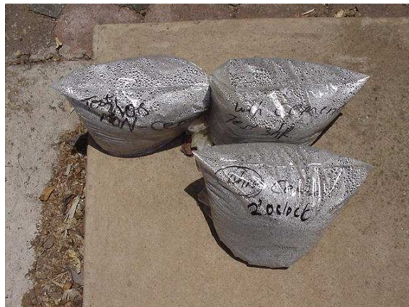
Photograph 7: Modified AASHTO samples exposed to site conditions before compaction
