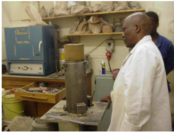
Photograph 5: Extruding the 4 hour Builtcrete sample after compaction on the vibratory compaction table.
