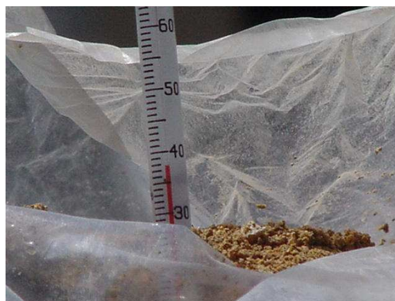
Photograph 1: temperature inside Builtcrete sample just before compaction
