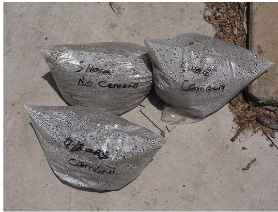
Photograph 8: Vibratory table samples exposed to site conditions before compaction
