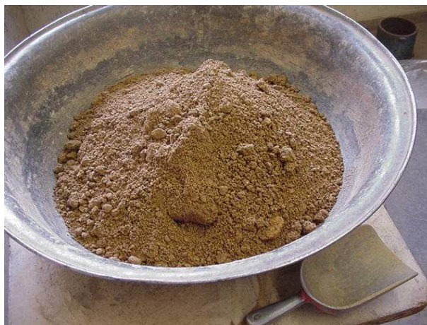
Photograph 4: Four hour Builtcrete treated material just before compaction. Notice more lumpy appearance.
