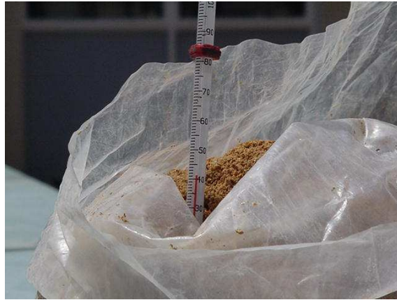
Photograph 2: Temperature inside lime/slag sample just before compaction The temperatures were very similar for both stabilized materials.
