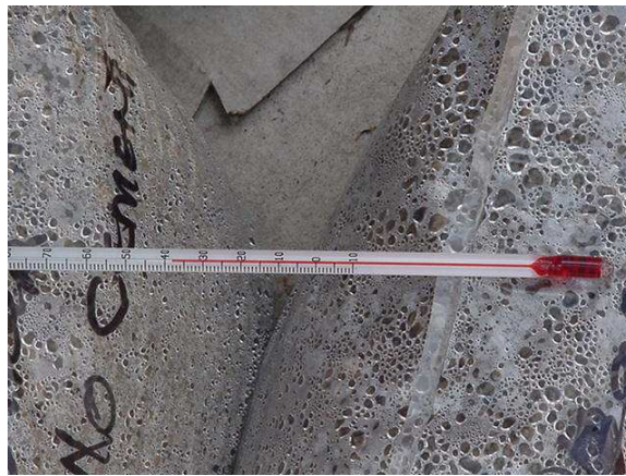
Photograph 9: Temperature measurement on top of samples showing temperature
