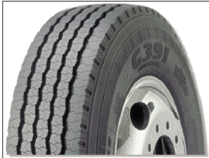
Figure 1: Image of the type 12R22.5 HVS Mk IV + single test tyre (Normally, the HVS test use a dual tyre set)
