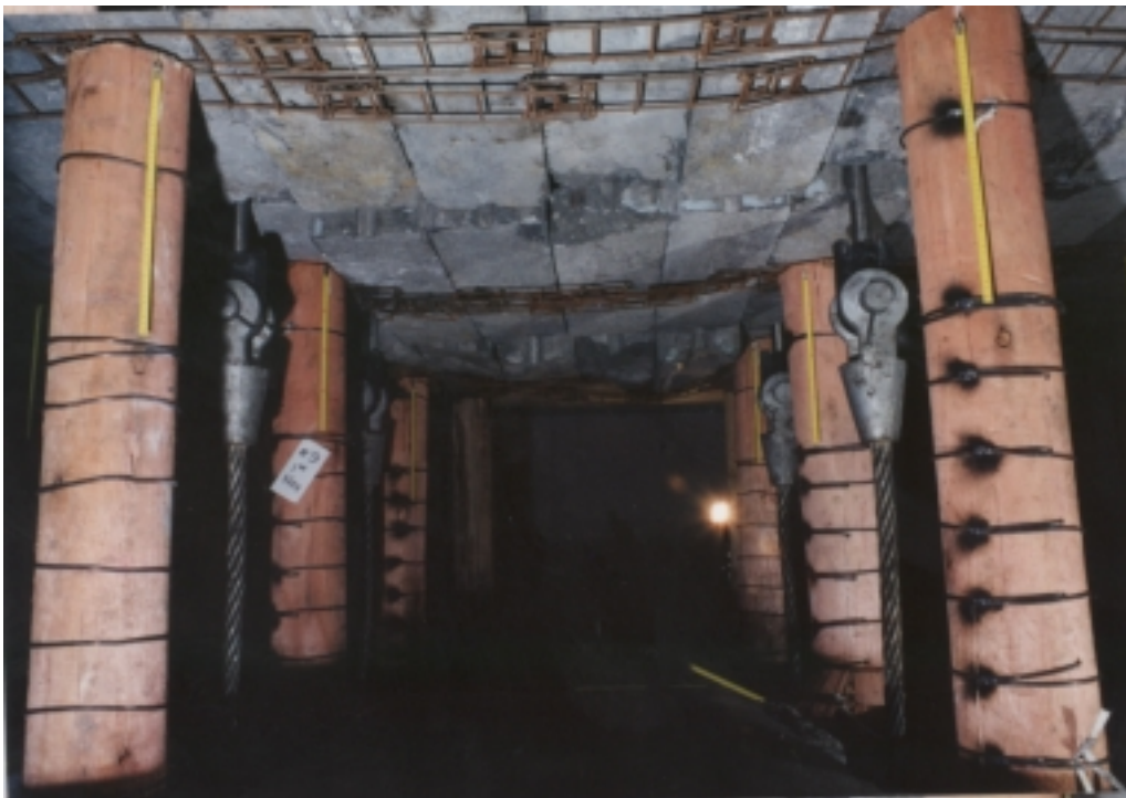
Photograph 5.17 Test # 9 showing en masse movement of centre four blocks after the first impulse of 83,5 kJ with no visible unfolding of Samson strap overlap.
