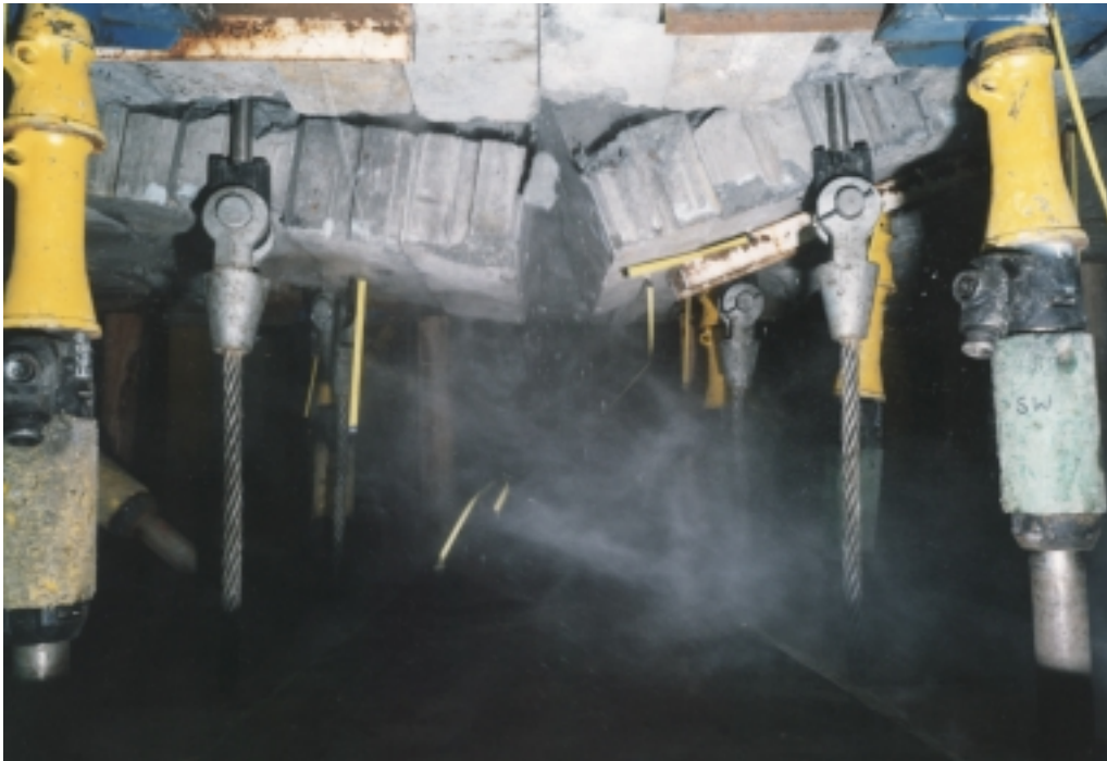
Photograph 5.9 Test # 3 approximately 50 milliseconds after impulse of 139 kJ with an impact velocity of 5,3 \text{ ms}^{-1} .
