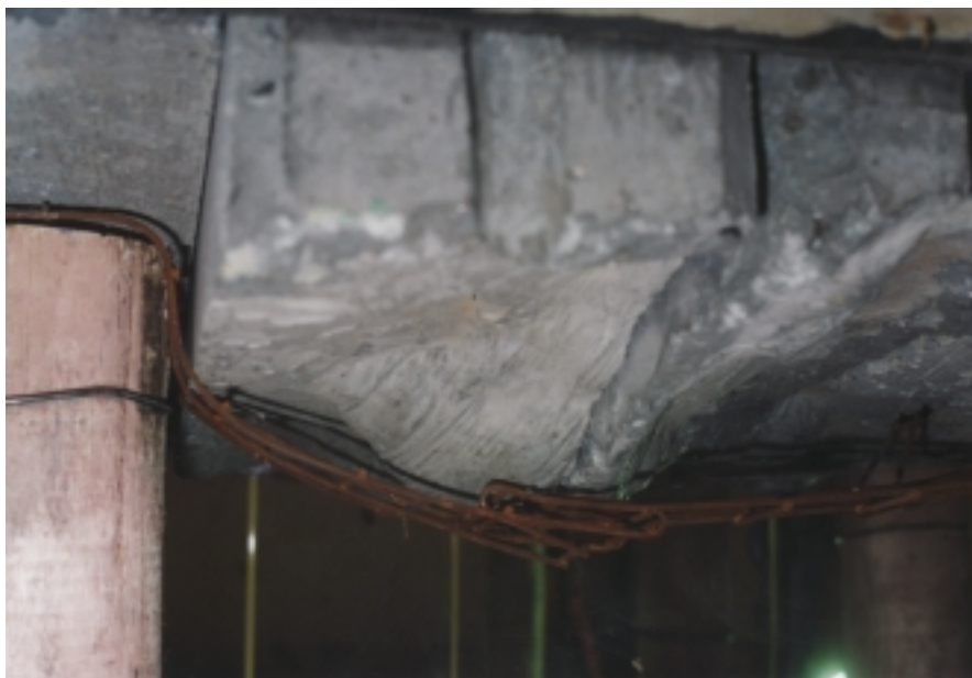
Photograph 5.13 Test # 7 showing 57 mm of step displacement at the southern prop and overlap starting to open.
