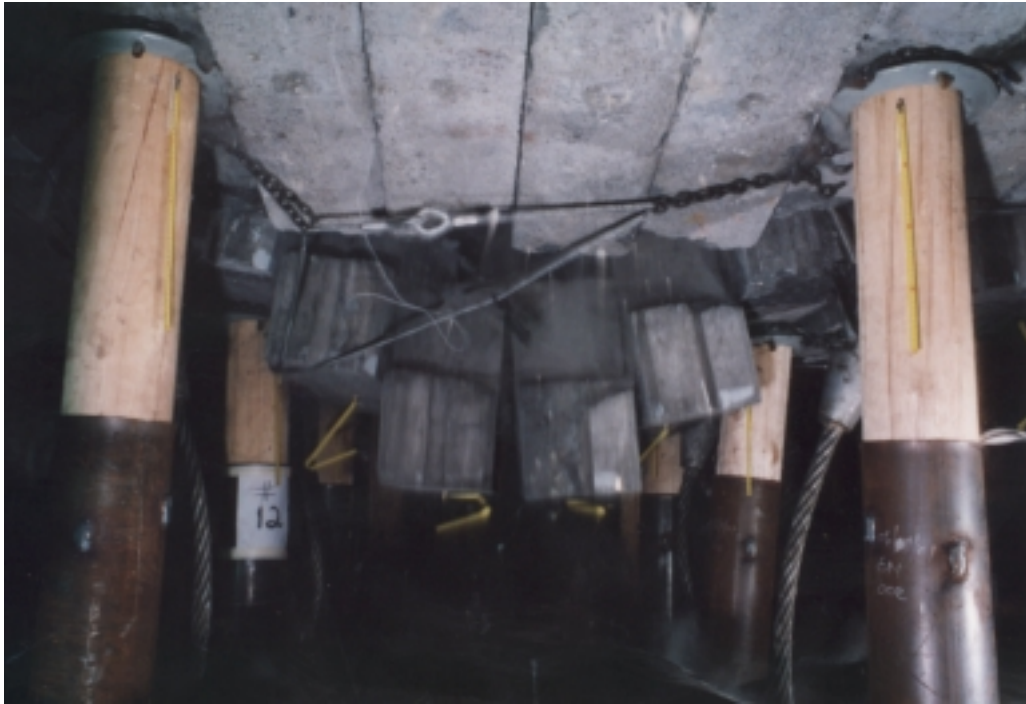
Photograph 5.24 Test # 12 shortly after impact of first impulse of 290 kJ at velocity of 7,5 ms -1 .
