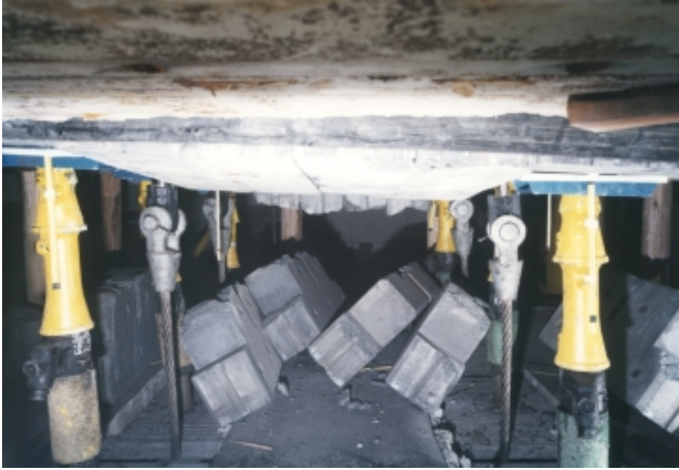
Photograph 5.5 Test # 1, all blocks collapsed except above each 400 mm headboard.
