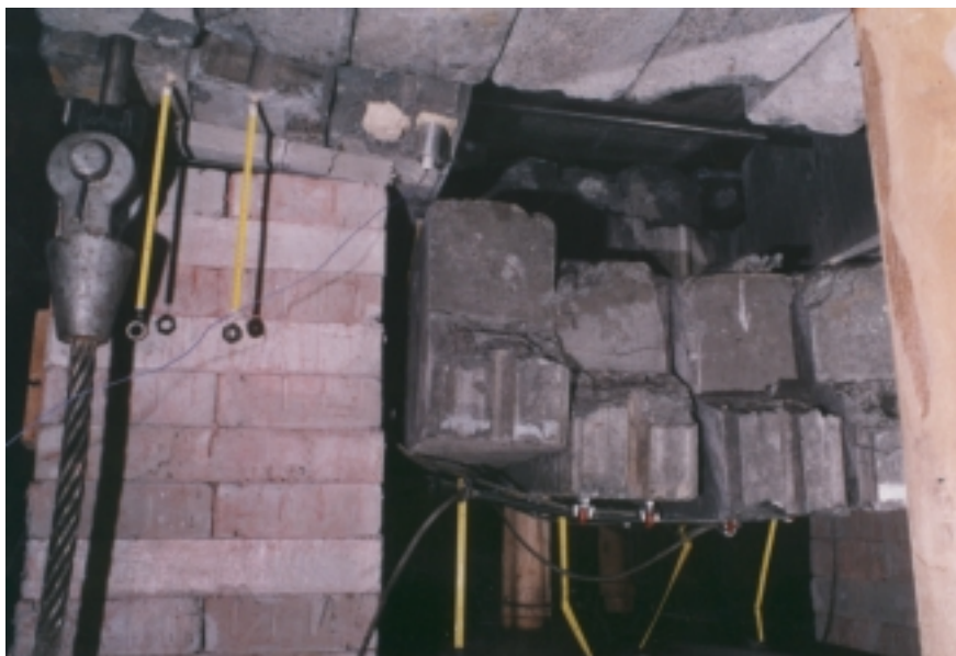
Photograph 5.30 Test # 13, showing arrested centre blocks.
