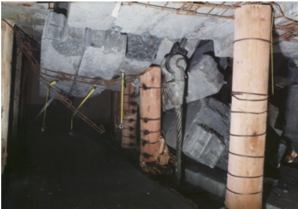
Photograph 5.18 Test # 9, after the second impulse of 196,4 kJ at an impact velocity of 6,2 \text{ ms}^{-1} . View of North elongate showing one Samson strap pulled open while the other appears to have helped support blocks 1, 2 and 3.
