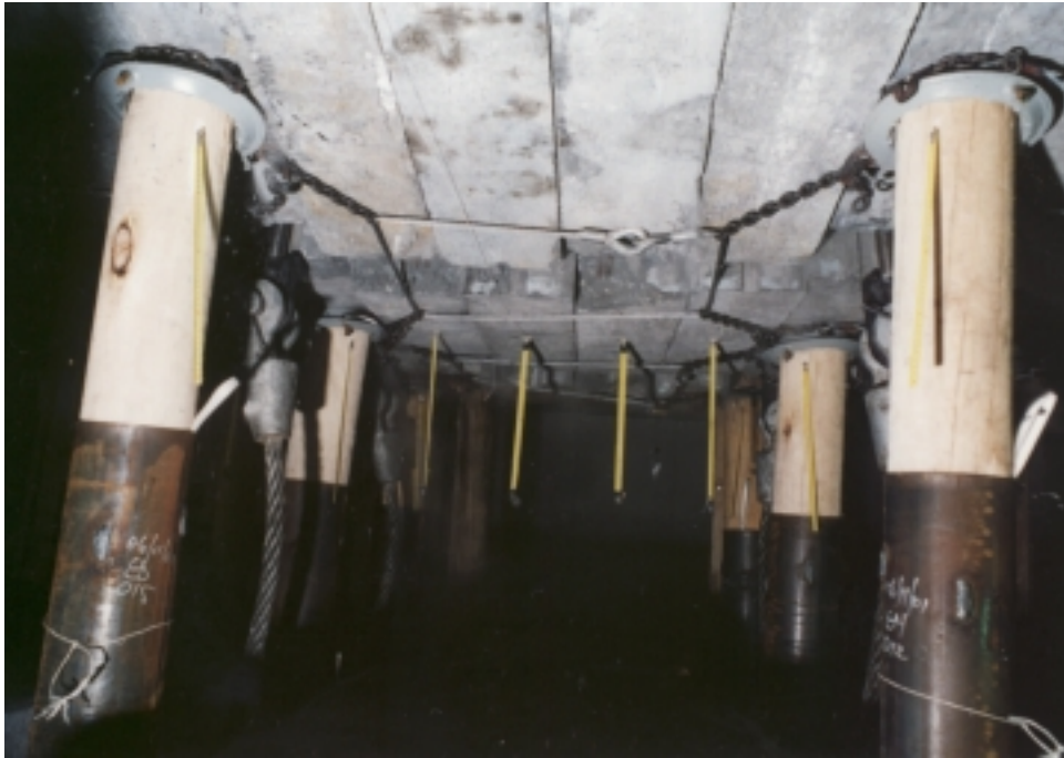
Photograph 5.20 Test # 10 shortly after impact of 88 kJ impulse at velocity of 4,2 \text{ ms}^{-1} .
