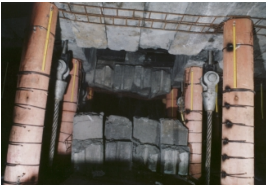
Photograph 5.16 Test # 8 indicating that Samson straps pulled apart at central overlap.
