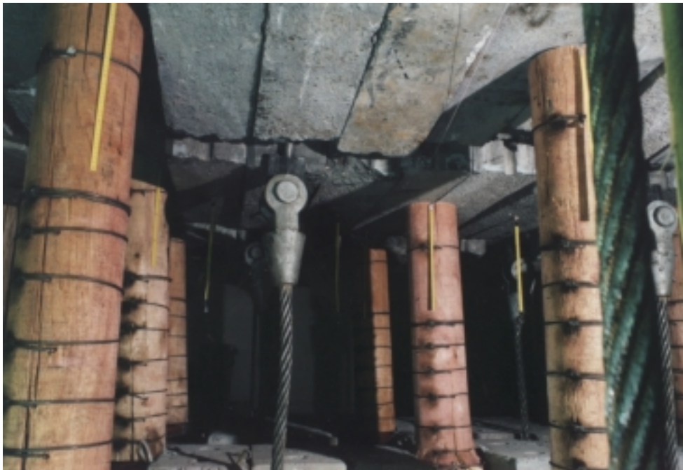
Photograph 5.3 Test # 5, after impulse of 147 kJ at impact velocity of 5,4 ms -1 showing 88 mm convergence on centre elongate.
