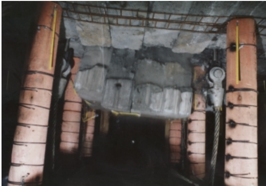
Photograph 5.15 Test # 8 some 200 milliseconds after impact of 147 kJ impulse at a velocity of 5,4 ms -1 .
