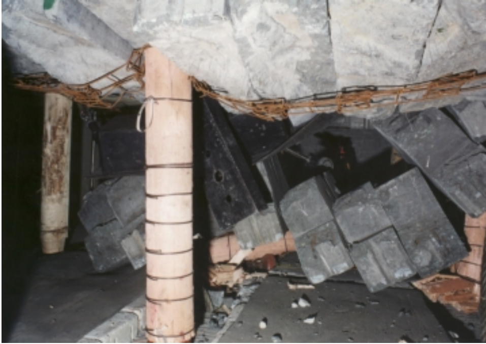
Photograph 5.19 Test # 9, after complete collapse resulted from asymmetrical ‘point-brush’ failure of base of North elongate.
