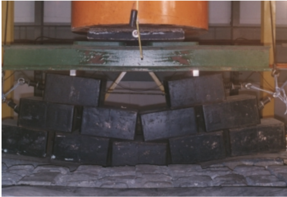
Photograph 5.31 Test # 13, showing disarrangement of two-dimensional pyramid after impact of 88,4 kJ.
