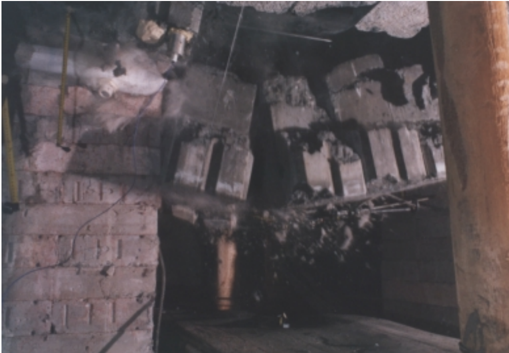
Photograph 5.34 Test # 14, shortly after impact of second impulse of 147,3 kJ at velocity of 5,4 \text{ ms}^{-1} . Accelerometer visible on block 4 gave velocity estimate of 3,3 \text{ ms}^{-1} .
