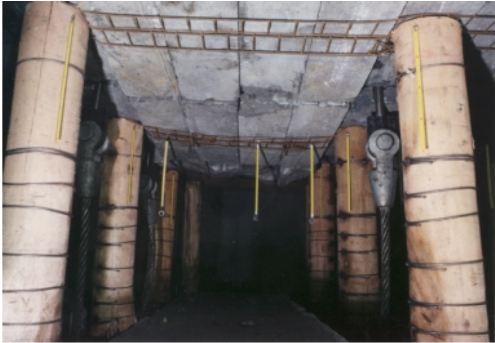
Photograph 5.12 Test # 7 after third impulse of 147 kJ at impact velocity of 5,4 \text{ ms}^{-1} .
