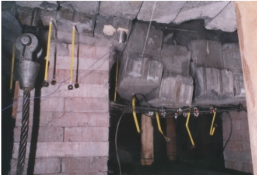
Photograph 5.29 Test # 13, shortly after impact of first impulse of 88,4 kJ at velocity of 4,2 ms -1 .
