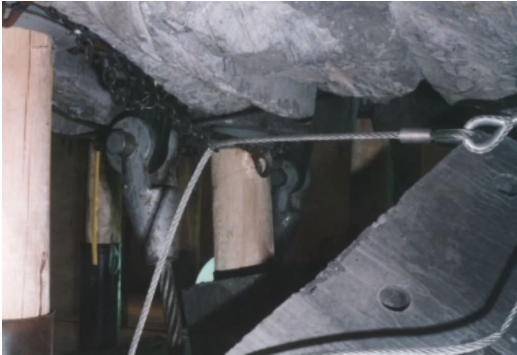
Photograph 5.26 Test # 12, close view of SE collar segment with 'button-hole' stretched open.
