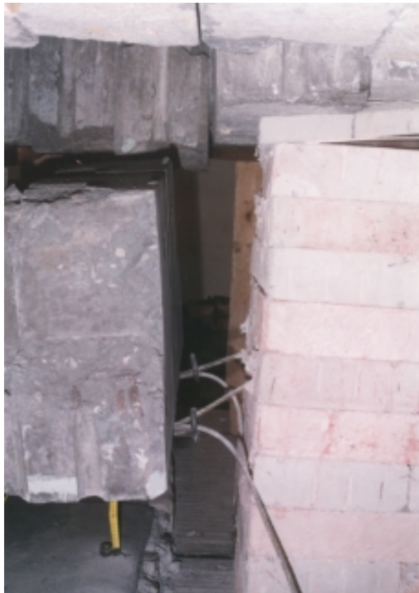
Photograph 5.27 Test # 13, showing tilted blocking layer of South pack.
