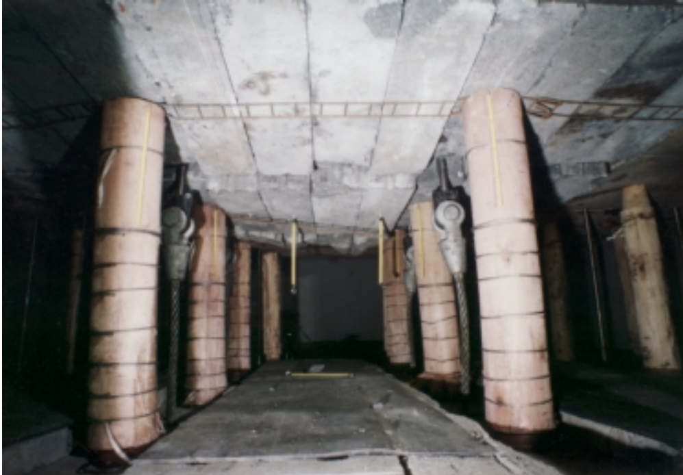
Photograph 5.11 Test # 6 after the second impulse of 88 kJ which impacted at a velocity of 4,3 ms -1 .
