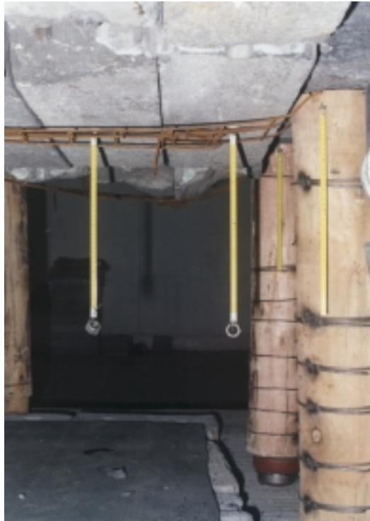
Photograph 5.13 Test # 7 showing 57 mm of step displacement at the southern prop and overlap starting to open.
