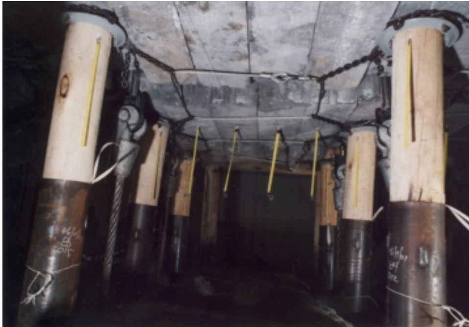
Photograph 5.21 Test # 10, shortly after second impulse of 147 kJ impacted at velocity of 5,4 ms -1 .
