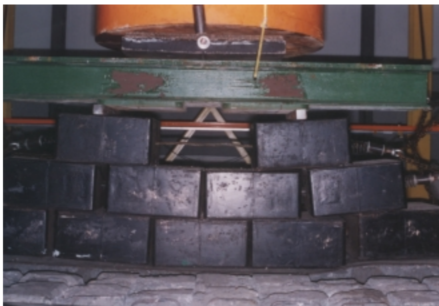
Photograph 5.33 Test # 14, showing relatively little disarrangement of load distribution pyramid after first impulse.
