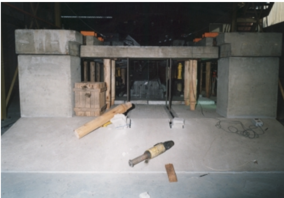
Photograph 5.10 Test # 3, showing collapse of centre Voussoir beam and dramatic ejection of northern prop.
