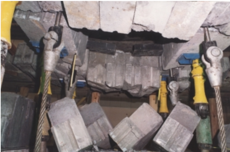
Photograph 5.6 Test # 1, showing significant sliding of centre four blocks in East beam and in West beam.
