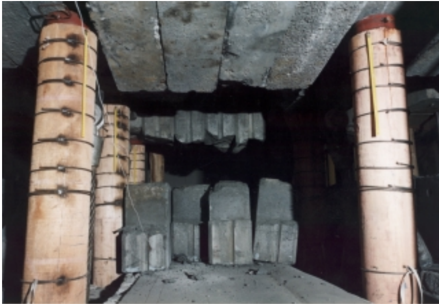
Photograph 5.1 Test # 4, approximately 50 milliseconds after impulse of 147 kJ at impact velocity of 5,4 ms -1
