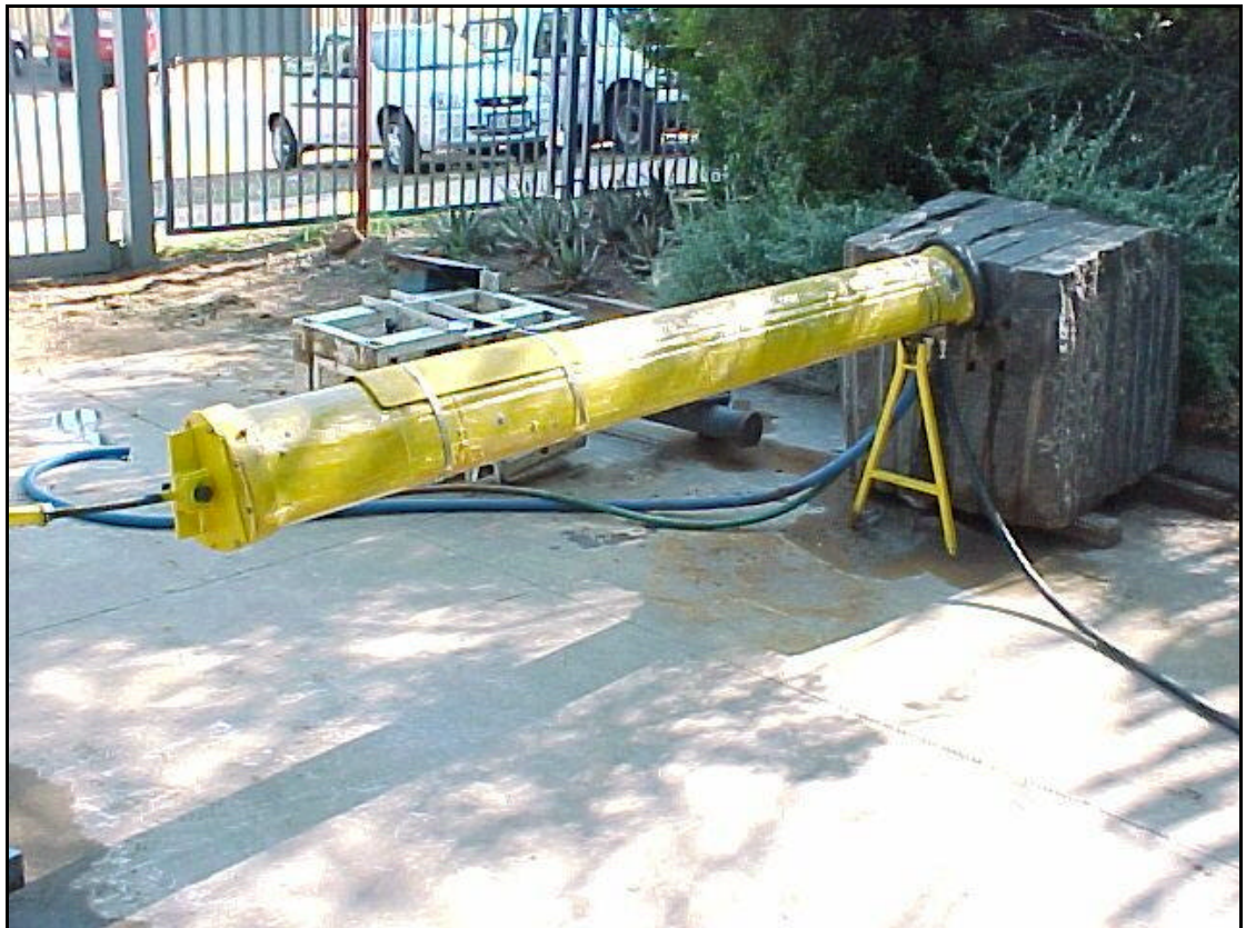
Figure 9-1: Photo of the quiet rock drill drilling into a granite block
