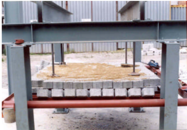
Figure A.1. Preparation of bricks assembly.
