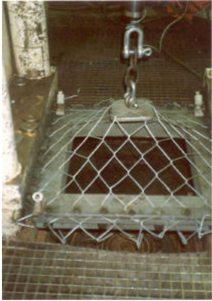
Figure A.57. Pull test diamond mesh (B).
