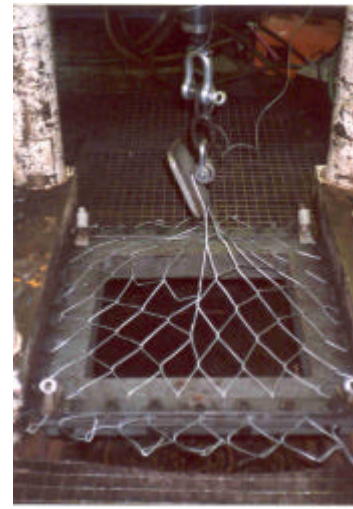
Figure A.55. Pull test diamond mesh (B).
