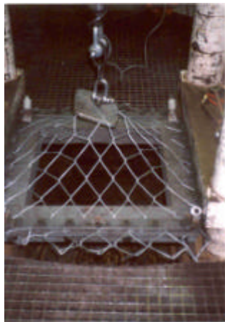
Figure A.54. Pull test diamond mesh (B).
