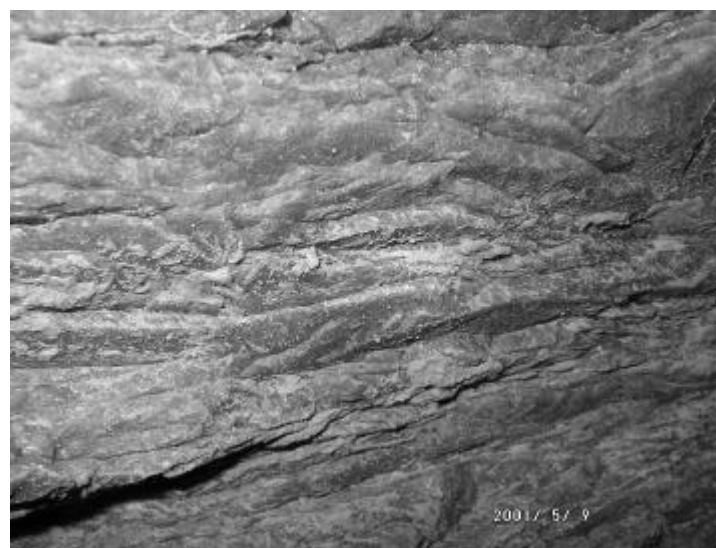
Figure 4.5.7 Photograph of shallow dipping fractures in 'window 3', (60 m from face) 50-25 E5 gully at Driefontein 5 Shaft
