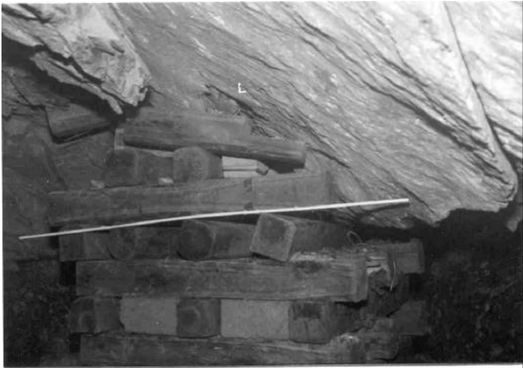
Figure 4.4.5 Hangingwall at top of E1 panel, 94-48 VCR stope at Mponeng mine (face at right)
