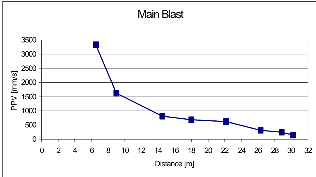
Figure 3.12 Attenuation curve of peak particle velocities measured from the main blast.
