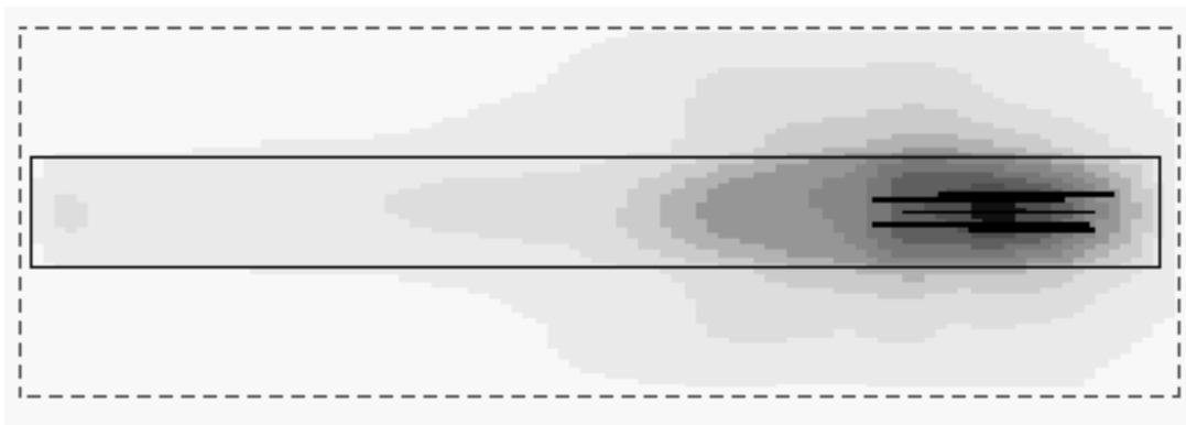
Figure 3.6 Maximum velocities at near tunnel wall for the post-blast model source #4. Maximum velocity for a blast pressure of 1 GPa is much lower than that recorded. Position of maximum velocity is now opposite the blast holes, due to the relatively long wavelength, and synchronisation of the blasts.
