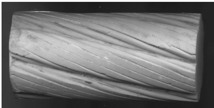
Figure D4.1: A well deformed triangular strand rope.
