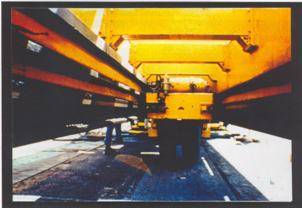
PHOTOGRAPH A.4 : The test carriage fitted with a dual truck wheel
