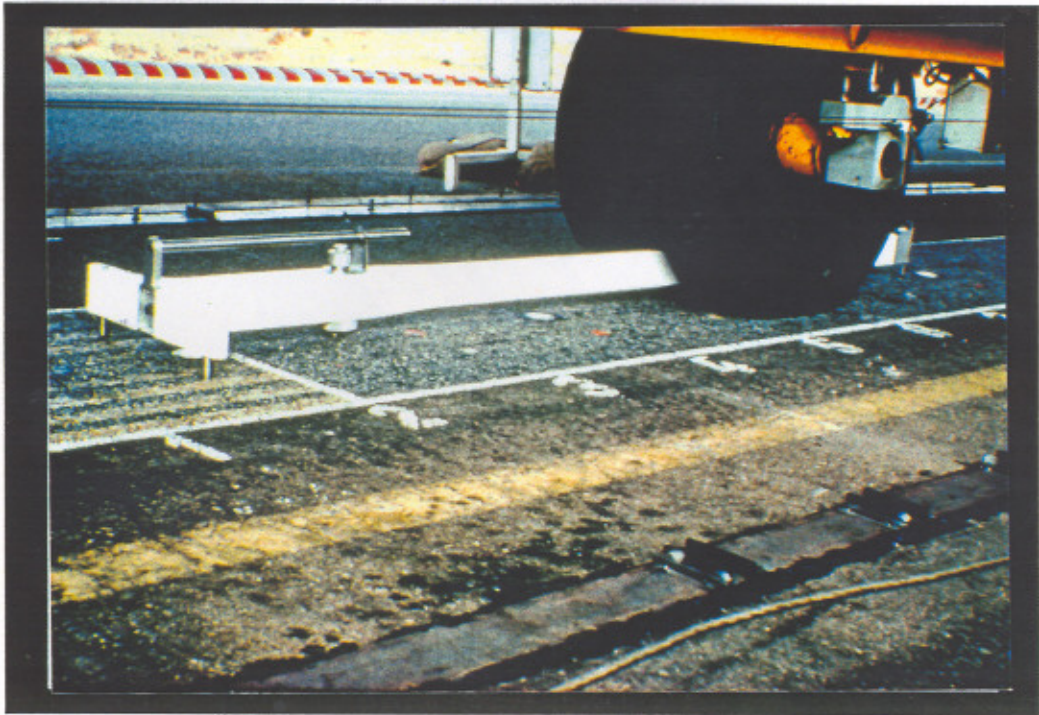
PHOTOGRAPH A.6 : The Road Surface Deflectometer (RSD)
