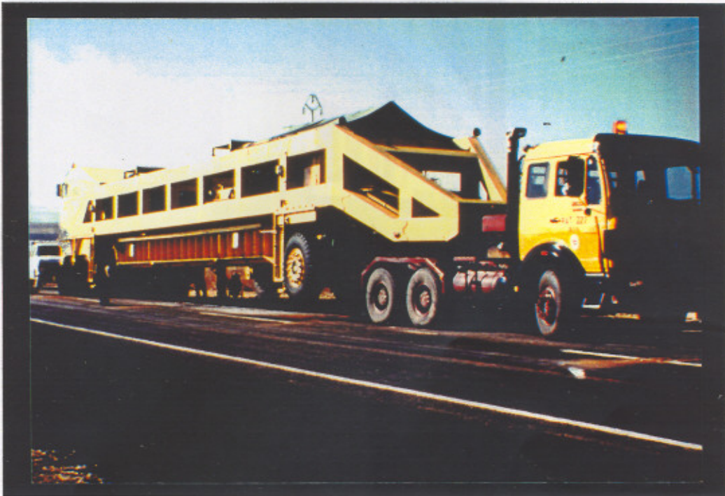
PHOTOGRAPH A.3 : Long distance hauling of the HVS using a tractor
