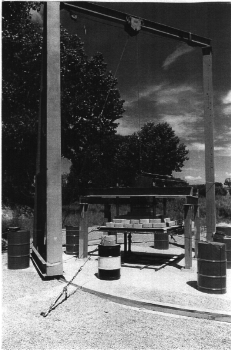
Photo 4: View of suspension of drop weight from overhead trolley.
