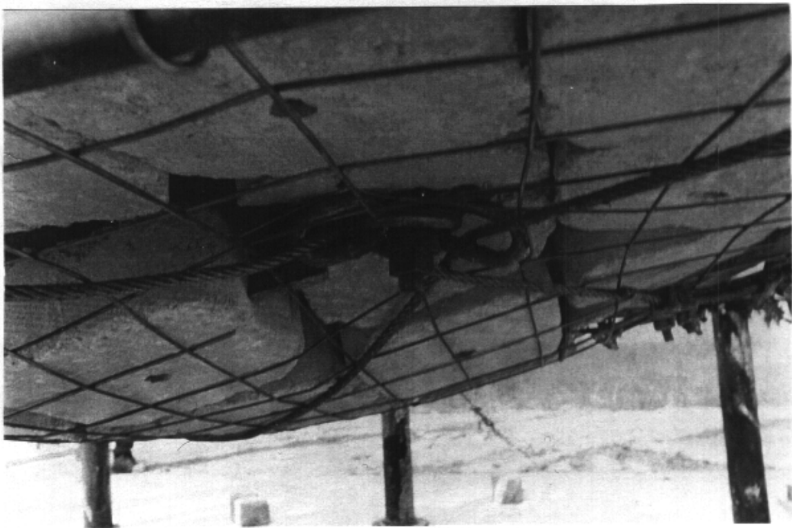
Photo 18: Test No. 39. Impulse 37 kJ, deflection 211 mm. 100 x 3,5 weld mesh was backed by 10 mm lacing connected to rock bolts by 3-link chain-link connectors.
