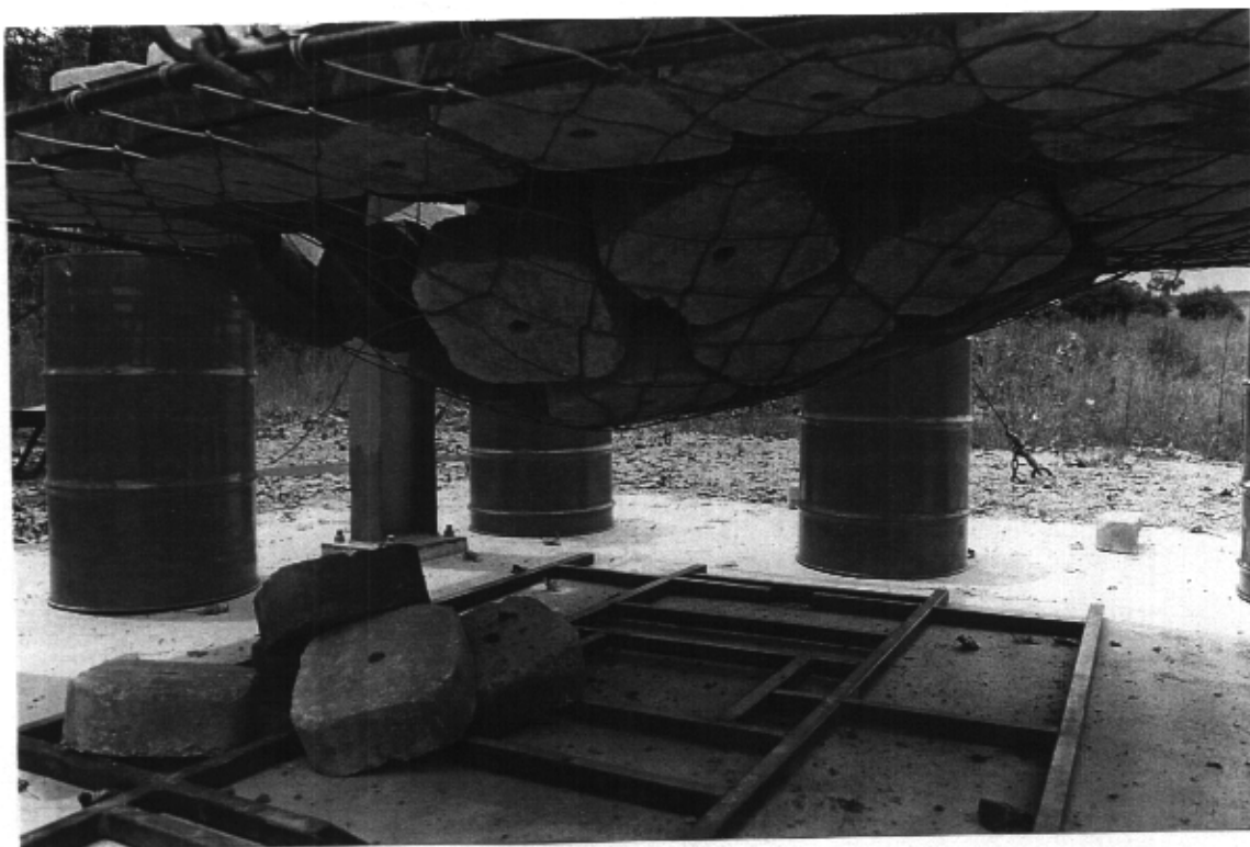
Photo 6: Test No. 7. Impulse 12,1 kJ, 246 mm deflection. View of underneath of diamond mesh test specimen showing unravelling at N-W corner and five blocks spilled.
