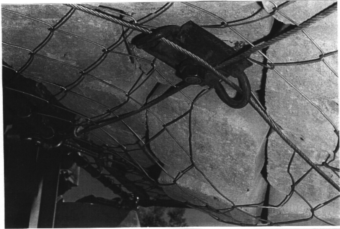
Photo 17: Test No. 31. Impulse 32,9 kJ, 176 mm deflection. Use of 'eared' lacing-plates has prevented damage to 8 mm lacing. Unravelling of diamond mesh has commenced but no brick spilled.
