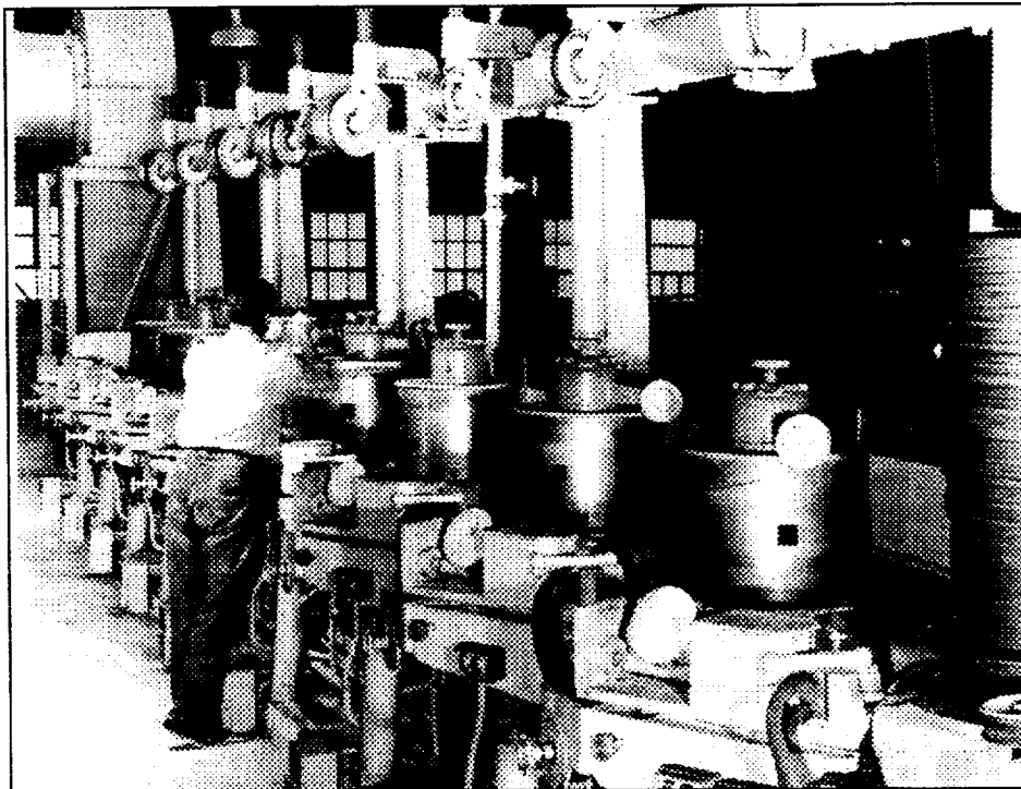
Figure 36 Overhead Take-off Wire Drawing Machine
