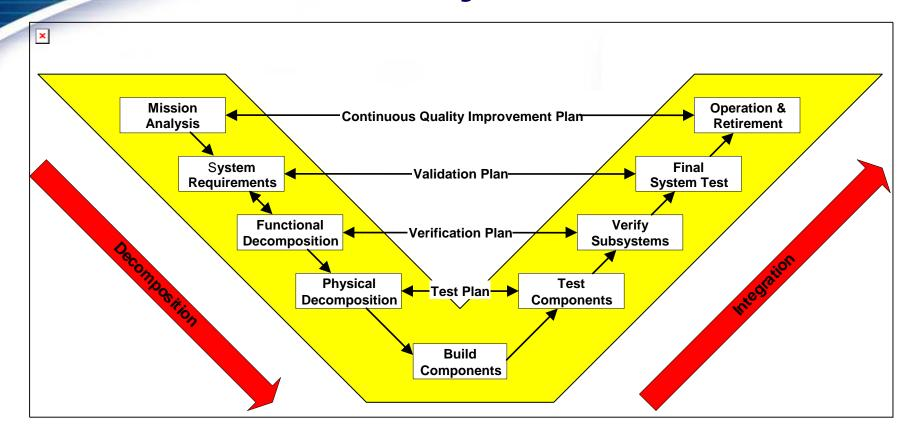
The design downstroke and the manufacturing upstroke
