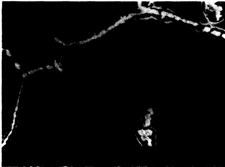
Fig. 4 \gamma' and carbide morphology after creep to 8\dot{\epsilon}_m and then given the high temperature anneal (16hrs 1323K, AC, 16hrs 1123K, AC).
