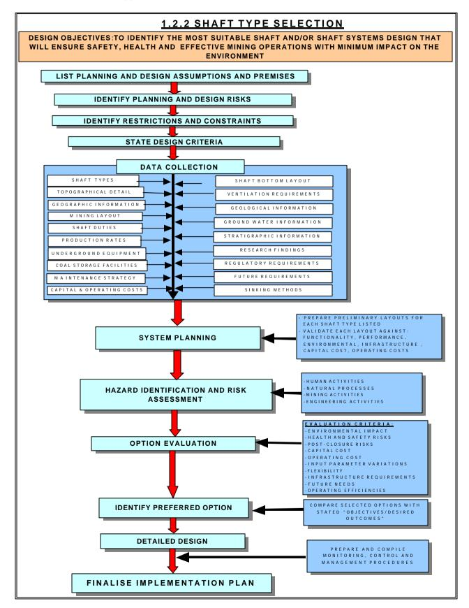
**<u>Objectives/desired outcomes</u>**: To identify the most suitable shaft system design for a specific coal deposit that will ensure the safety and health of employees, will ensure an effective mining operation and have minimum impacts on the environment.
