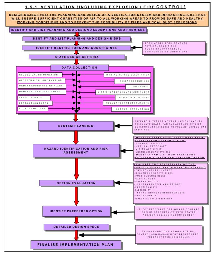
**Objective/desired outcomes** The planning and design of a mine ventilation system, associated infrastructure and control mechanisms that will ensure the effective supply of sufficient quantities of air to the designated underground working areas for the purposes of providing safe and healthy working conditions and for the prevention of underground fires and coal dust explosions.
