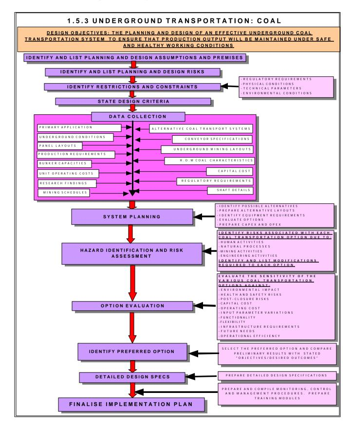
**<u>Objectives/desired outcomes</u>**: To plan and design an effective underground coal transportation system to ensure that the required output rates from the various production sections can be maintained over the life cycle of the mine under safe and healthy operating conditions, within the constraints of prevailing geological conditions, the prescribed mining plan and production schedules.
