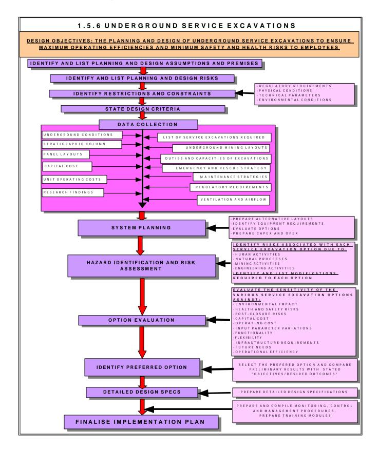
**<u>Objectives/desired outcomes</u>**: To plan and design the necessary service excavations (e.g. workshops, pump chambers, rescue bays, coal bunkers, underground stores, etc.) that will be required for a specific underground coal mining operation to ensure maximum operating efficiencies with minimum health, safety and environmental risks.
