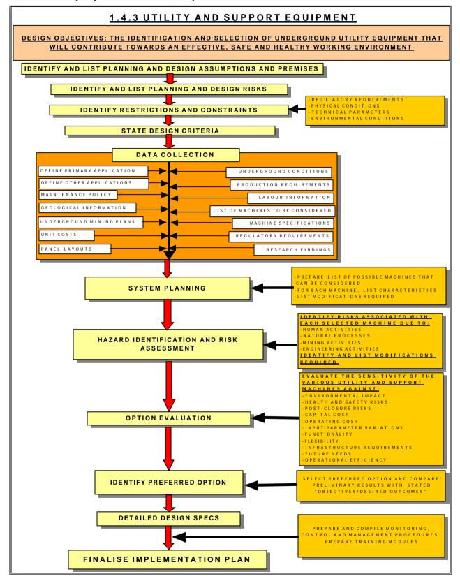
**Objectives/desired outcomes:** The selection and specification of the type and number of trackless underground utility and support machines which, if properly complied with and implemented, will contribute towards achieving improved health, safety and production standards and conditions in the planned underground mine.
