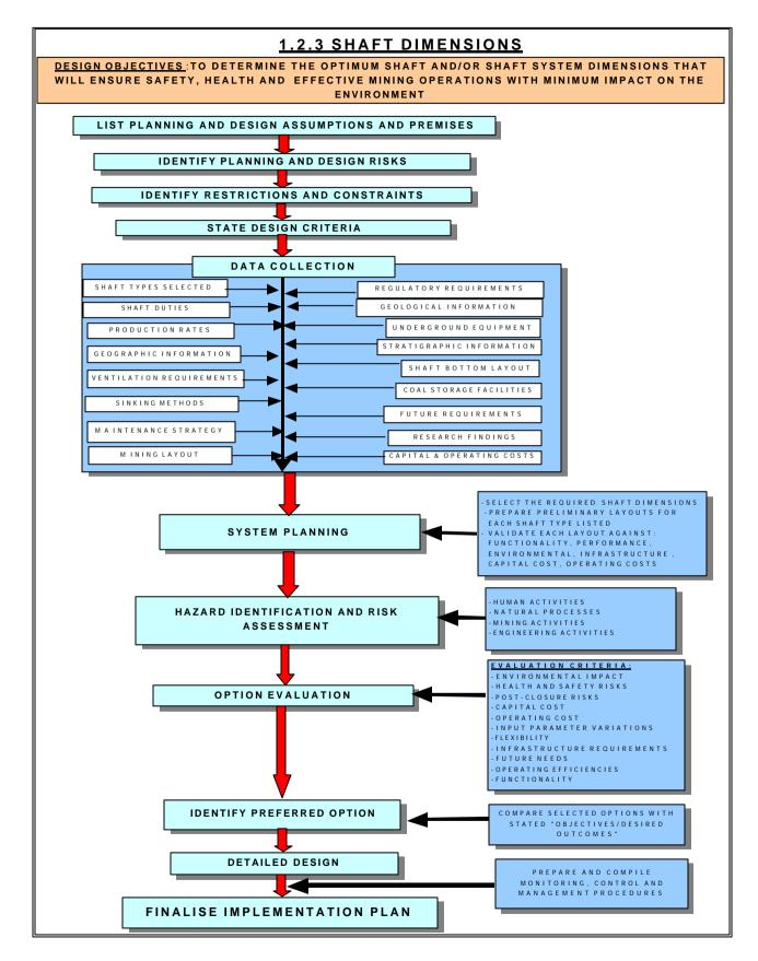
**<u>Objectives/desired outcomes</u>**: To determine the optimum shaft dimensions for a specific underground coal mining operation in order to provide cost-effective operating conditions complying with acceptable health, safety and environmental standards.
