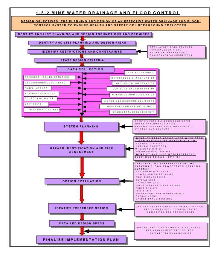
**<u>Objective/desired outcomes</u>** The planning and design of an effective mine water drainage and flood-control system that will ensure the health and safety of all underground employees and the protection of mine workings and equipment.
