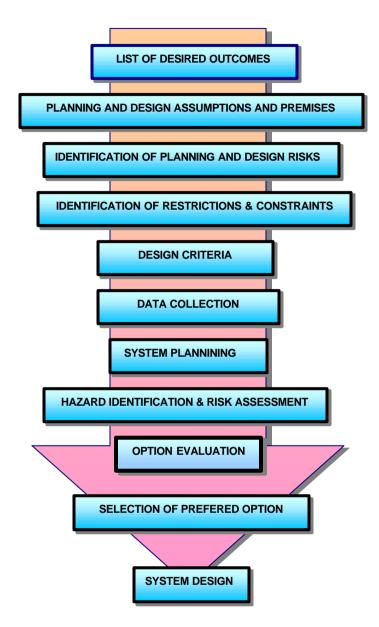
During the initial phases of any mine planning and design study, a number of assumptions and premises have to be made and accepted. As the planning and design process progresses from one phase to another, the amount of relevant data available for evaluation purposes increases, resulting in a corresponding increase in the confidence and accuracy level of the relevant mining plan.
