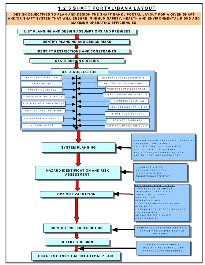
**<u>Objectives/desired outcomes</u>**: To plan and design the shaft portal/bank layout for a given shaft and/or shaft system that will ensure minimum health, safety and environmental risks and maximum operating efficiencies.
