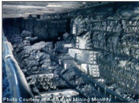
Figure 2.2 Coal plough in operation (Source: Australian Mining Monthly)
