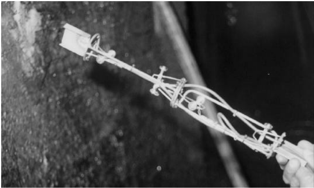
Figure 4–4 Vibrating wire cage with four vibrating wire gauges ready to be installed and grouted into the hole.
