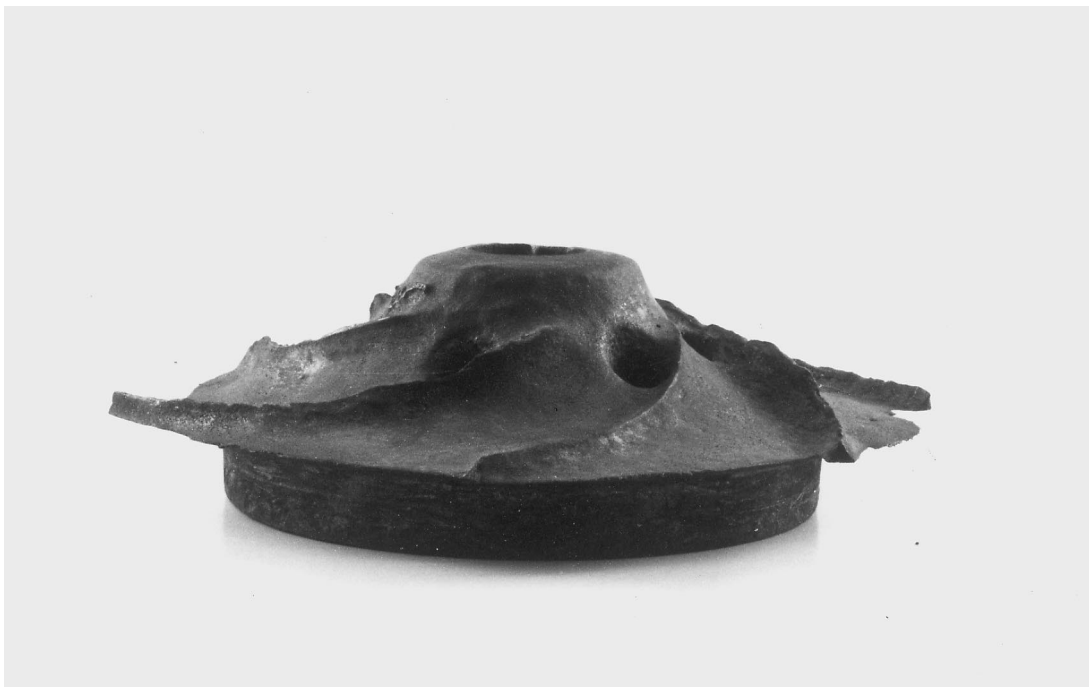
Fig. 9. General corrosion of a cast-iron impeller.
