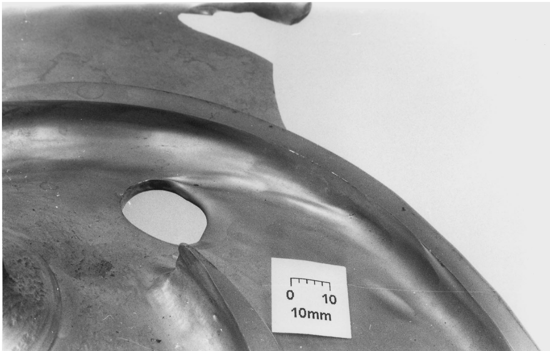
Fig. 10. Erosion–corrosion grooves and depressions on an impeller surface.
