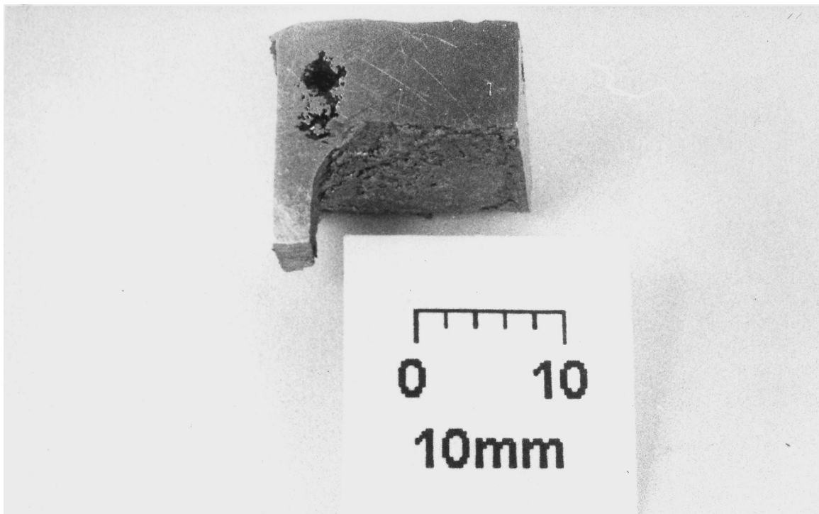
Fig. 2. Porosity on a cross section from the cracked region of Fig. 1.
