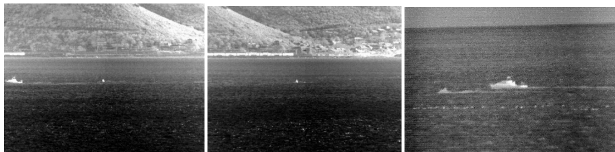
Figure 8: Small harbour patrol boat and jetski (left), Jetski (middle) both at 2 km, 3-5 \mu\text{m} in a highly cluttered coastal background; Jetski and small harbour patrol boat with wakes and birds in a sea background 8-12 \mu\text{m} .
