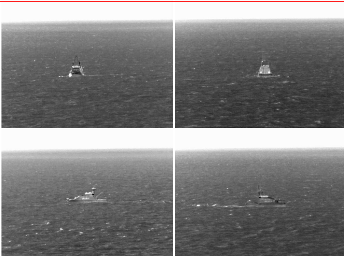
Figure 3: The small scientific work boat recorded in the 3-5 \mu\text{m} band at a distance of 1km (bow-upper left, stern-upper right, port-lower left, and starboard-lower right).
