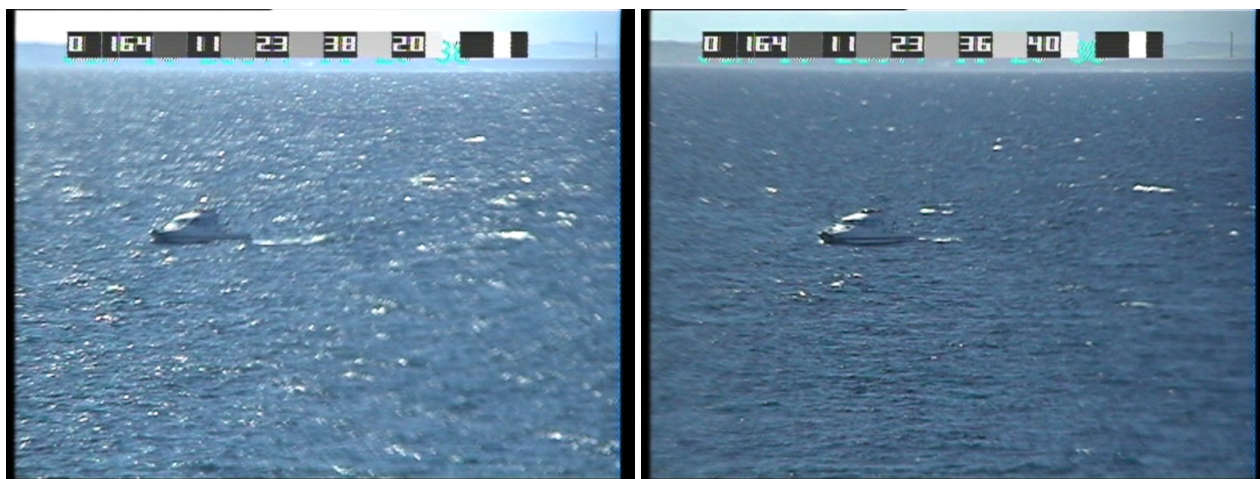
Figure 9: Visible light polarisation imagery of the small scientific work boat. Left horizontal, right vertical polarisation.
