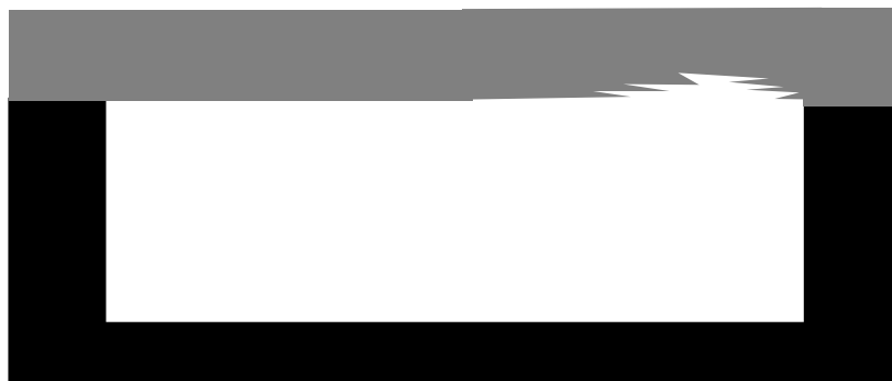
Figure 20. Guttering, caused by failure of the roof in horizontal compression.
