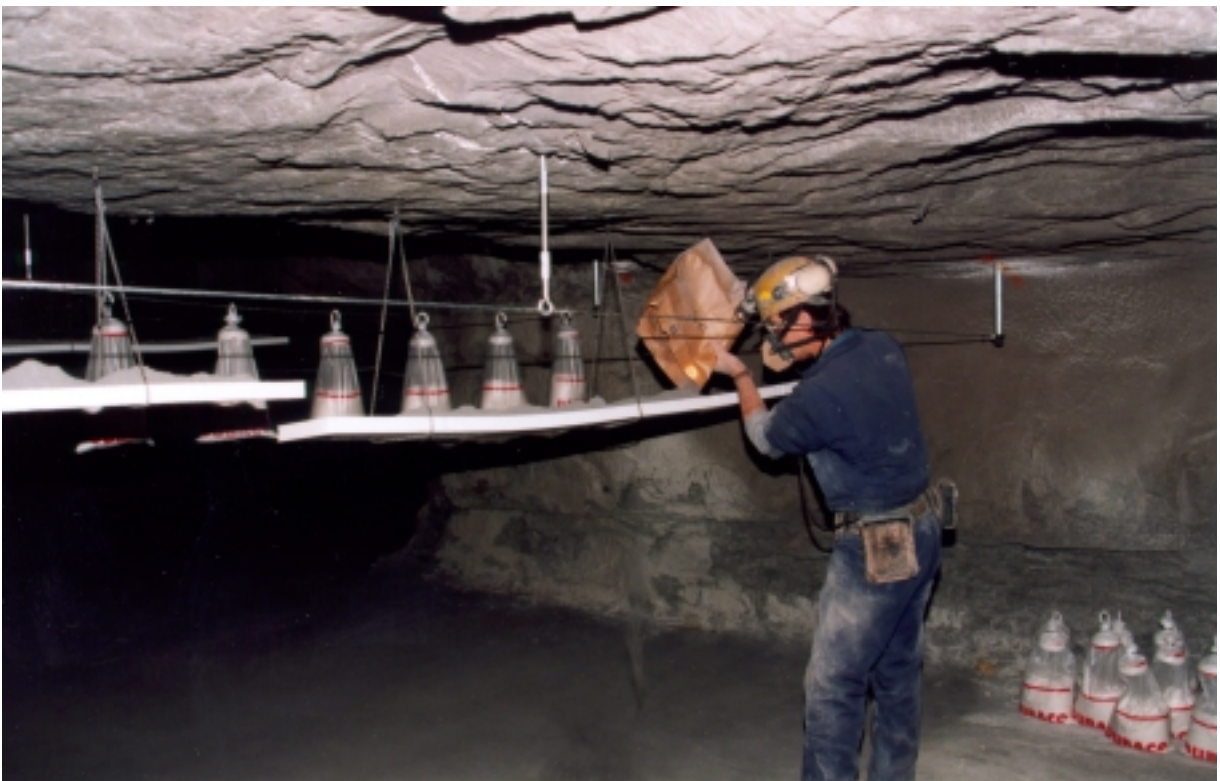
Figure 5.2.1b: Photograph showing coal dust distribution on shelves
