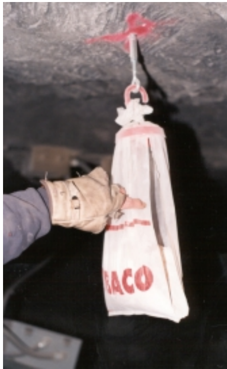
Figure 5.3.1.3a: Post-explosion photograph of a split bag
