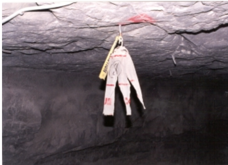
Figure 5.3.1.3b: Post-explosion photograph of an emptied bag
