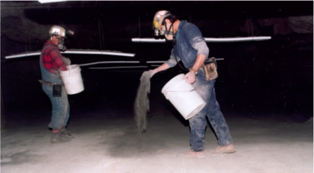
Figure 5.2.1a: Photograph showing coal dust distribution on floor
