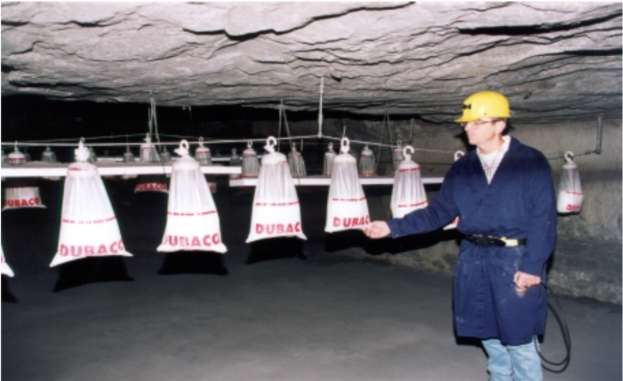
Figure 5.2.3a: Distributed barrier layout in B-drift
