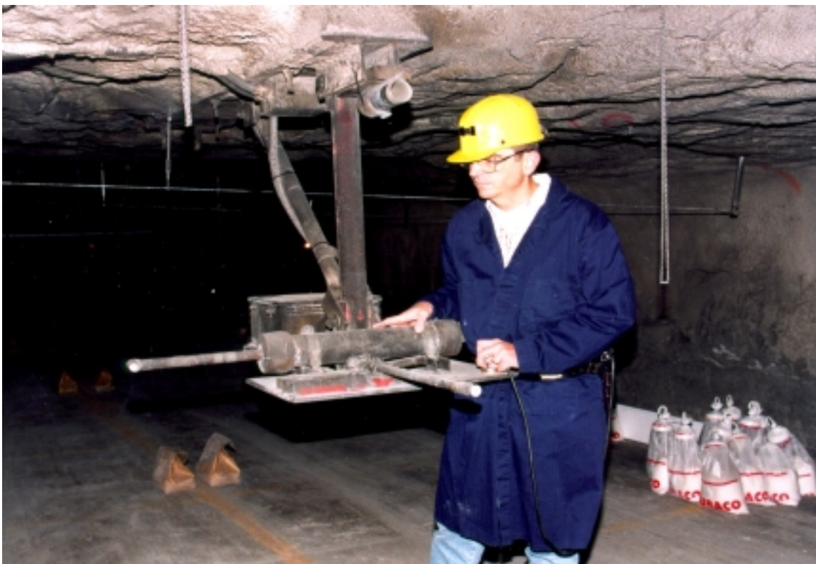
Figure 3.2: Instrument stand with the two different dynamic pressure instruments
