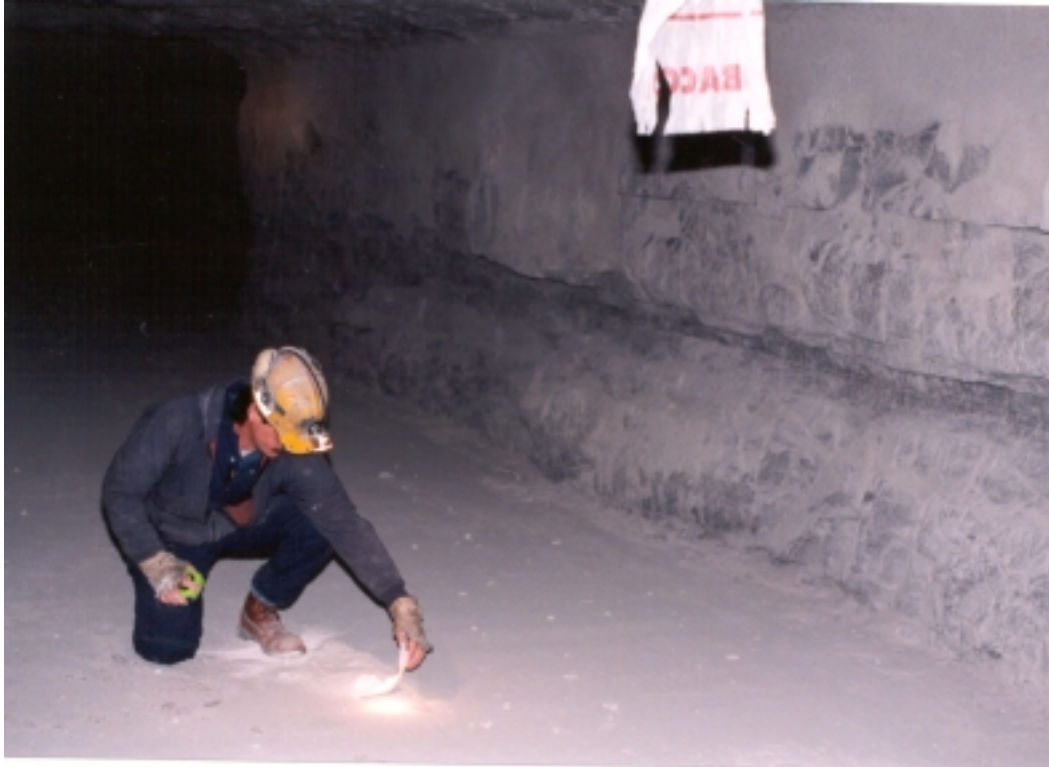
Figure 5.3.1.3c: Post-explosion photograph showing an emptied bag still suspended from the mine roof and technician estimating dust deposition on the outbye mine floor
