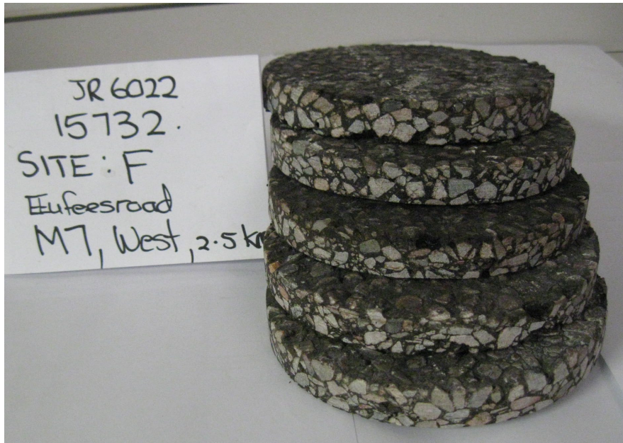
Figure 4: Cores taken from Eeufees Road (Site 8)
