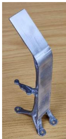
Fig. 6: Printed part in AlSi10Mg
