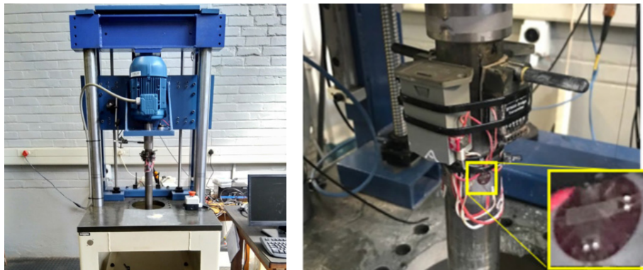
Figure 4. Laboratory rig used to develop drilling control system.
