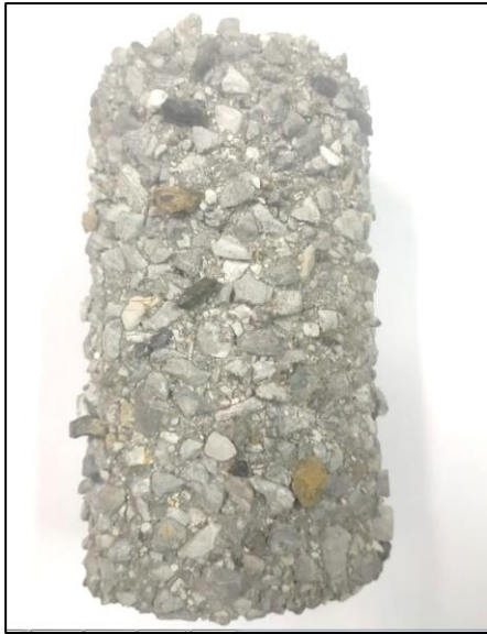
Figure 4-3 : CAC-dolomite specimen taken after 48 hours in the dynamic HCl test
