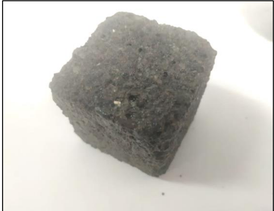
Figure 4-1 : CAC-dolomite specimen taken from the static HCl test after 350 hours
