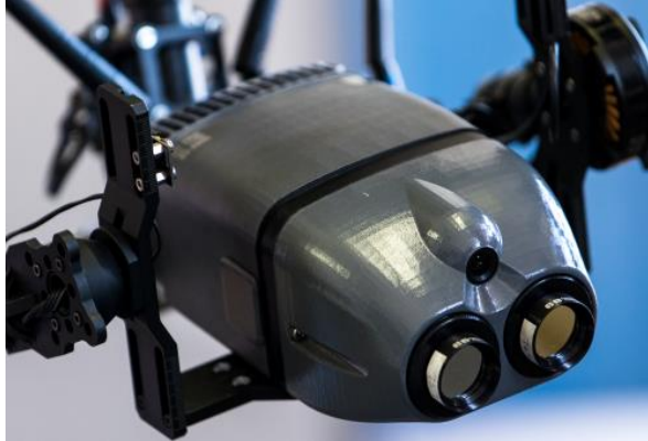
Figure 3: A closer look at the NIR sensor with two CMOS optical sensors placed side by side and furnished with ultra-narrow filters. A third wide field-of-view visible camera is also inserted and placed above the two cameras.
