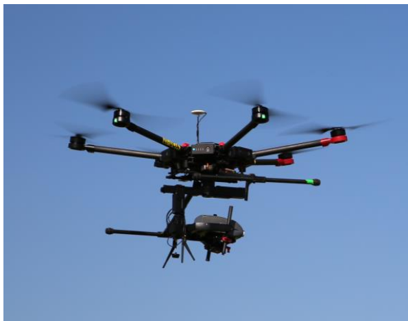
Figure 6: UAV with NIR sensor payload on the DJI 600 drone during a field fire detection test of the sensor.
