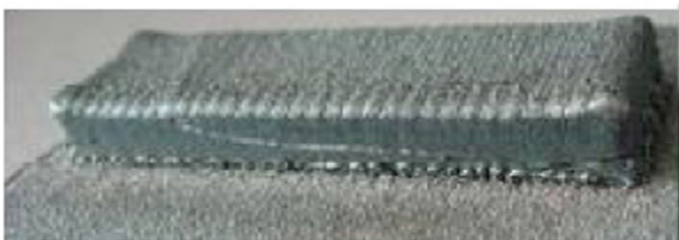
Fig. 6 During the DED deposition of Stellite alloys, cracking owing to residual stress occurred. Reproduced from Dutta., 2019. Metals: Science, Technology, and Additive Manufacturing Applications
