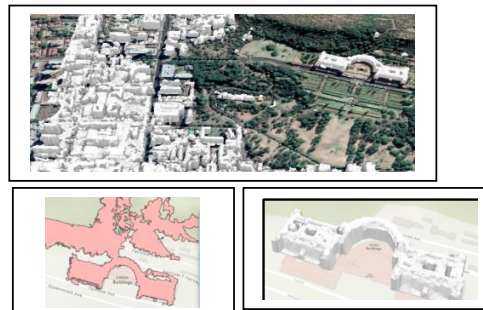
Figure 12. Post processing of footprints and solid models and Building Multipatch representing Digital Surface models of buildings as solid models
