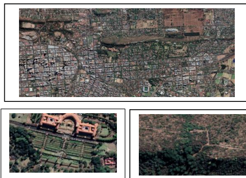
Figure 7. Orthoimage from ortho resampling. The orthophoto produced has very high resolution of 0.5m, good for ensuring georeferencing maintenance.
