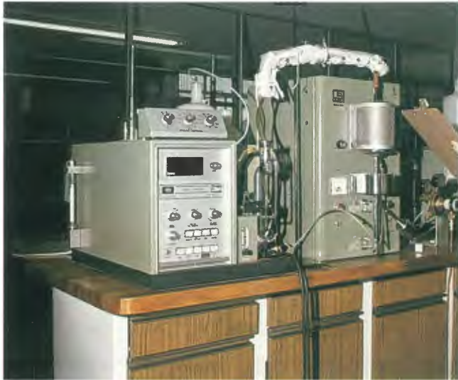
Sulphur determination in coal in LECO apparatus
