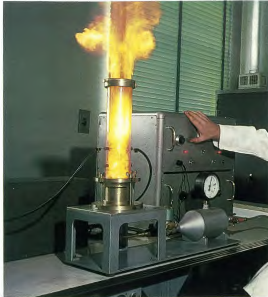
Explosibility of coal dust : Hartmann apparatus
