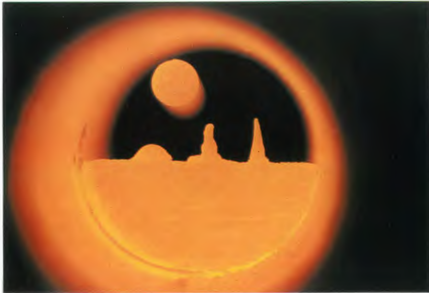
Ash Fusion Temperature : View into furnace showing samples at different levels of fusion
