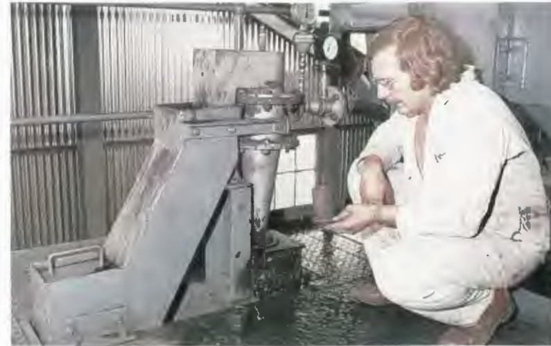
View of cyclone
