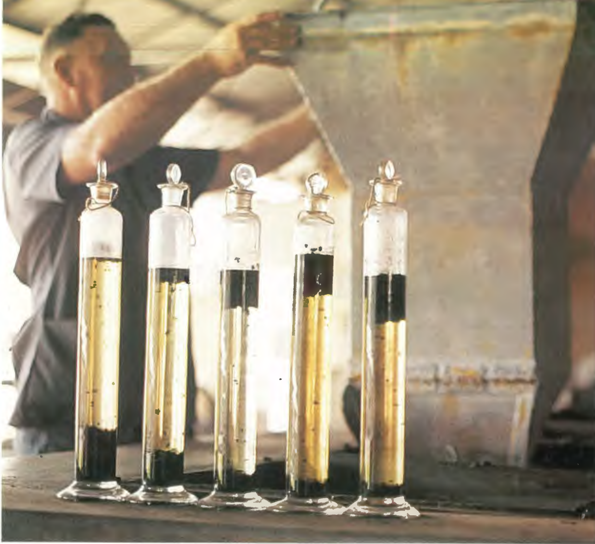
Float and sink analysis of coal
