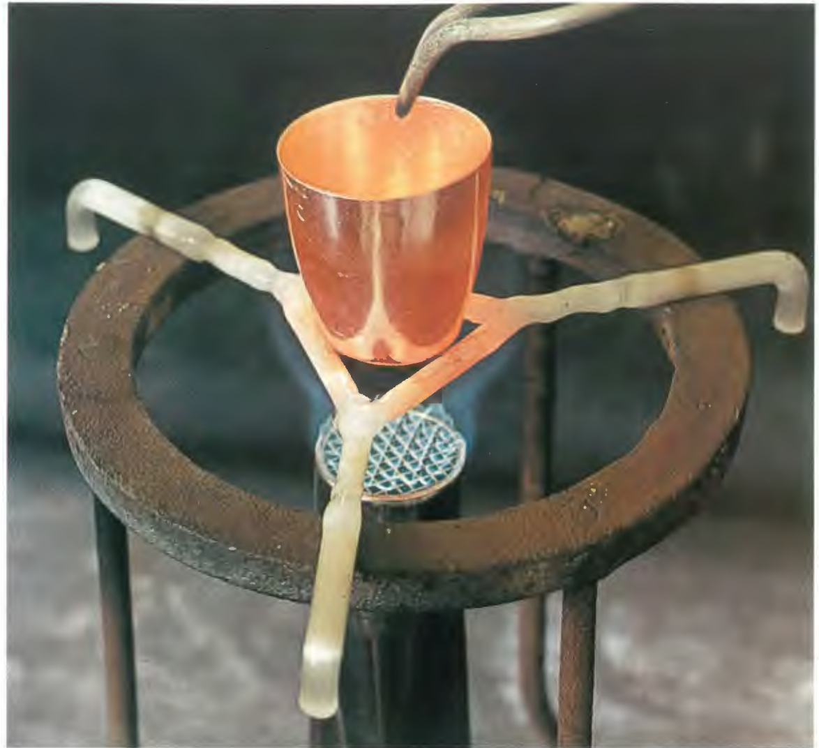
Coal ash being fused with fluxing agent in a platinum crucible
