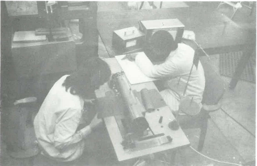
Testing the sewability of a cloth on a "Hattrasew" instrument recently acquired by the Clothing Technology Department
